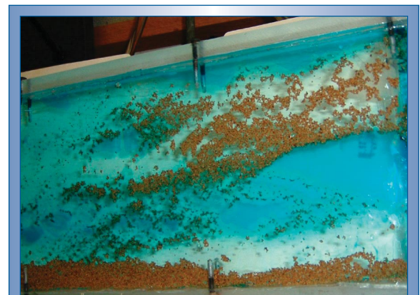
Figure 7. A slot-flow experiment showing proppant distribution in a reverse hybrid fracture treatment. The layers of gel created because of viscous fingering prevent settling of the proppant to the bottom of the fracture.
