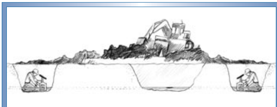
Figure 5. Conventional method for repairing large-diameter distribution lines.
