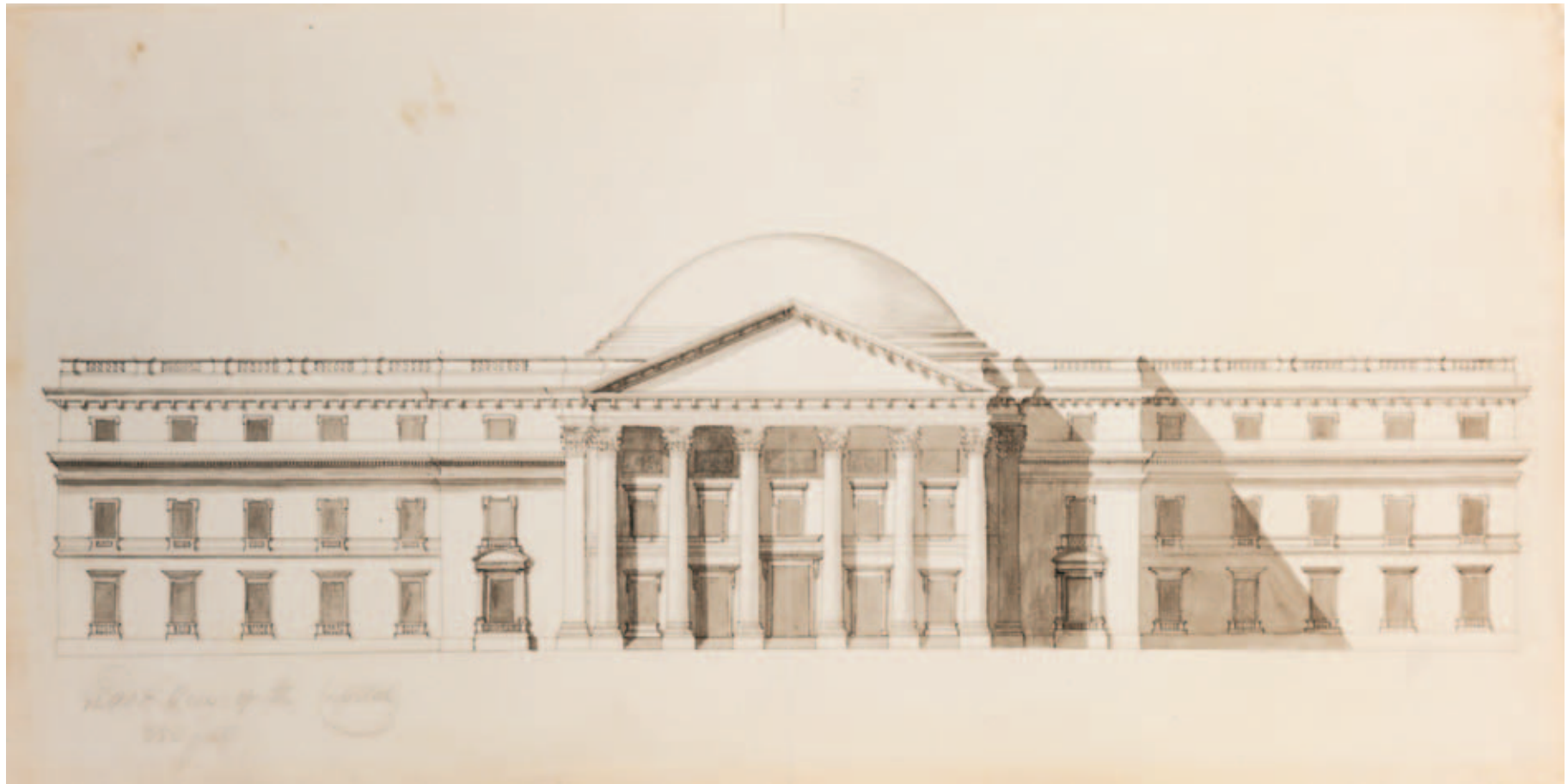
HALLET'S MODIFICATION OF THORNTON'S DESIGN, EAST ELEVATION. Unsigned drawing, ca. 1795, sometimes attributed to Hadfield, of the east front of the Capitol. MHS.
