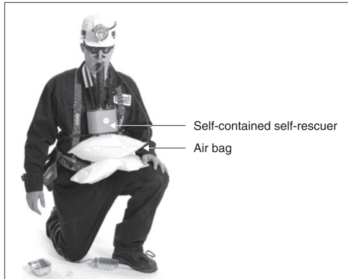
Figure 3: Example of Self-Contained Self-Rescuer That Provides Supplemental Air in Case of an Emergency
