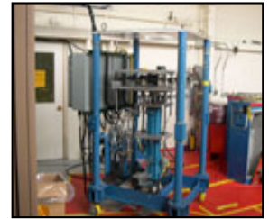
Planet, one of four CEF critical assemblies, is a vertical lift table-type critical assembly.
