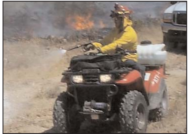
An All Terrain Vehicle conducts spot suppression and lays down a suppression line of fire retardant around NTS assets.
