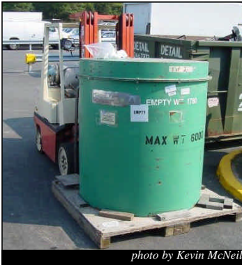
An overpack container is used to transport the sealed source unit to its final destination.
