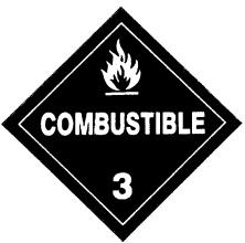
(b) In addition to complying with  $\S172.519$ , the background color on the COMBUSTIBLE placard must be red.
