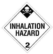
(b) In addition to complying with §172.519, the background on the POI-SON GAS placard and the symbol must be white. The background of the upper diamond must be black and the lower point of the upper diamond must be 65 mm (25% inches) above the horizontal center line. The text, class number, and inner border must be black.
