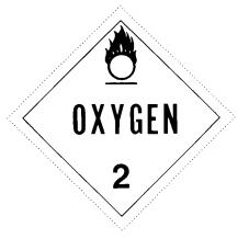
(b) In addition to complying with §172.519 of this subpart, the background color on the OXYGEN placard must be yellow. The symbol, text, class number and inner border must be black.
