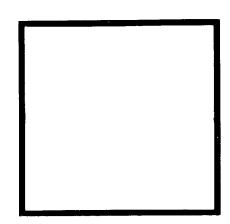
(b) In addition to meeting the requirements of \$172.519 for minimum durability and strength, the square background must consist of a white square measuring 14¼ inches (362.0 mm.) on each side surrounded by a black border extending to 15¼ inches (387.0 mm.) on each side.
