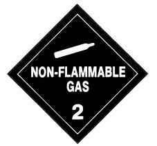
(b) In addition to complying with §172.519, the background color on the NON-FLAMMABLE GAS placard must be green. The letters in both words must be at least 38 mm (1.5 inches)
