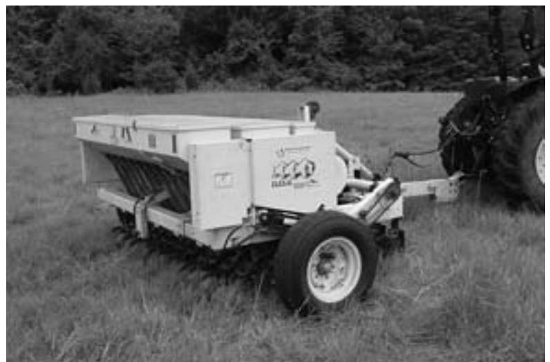
Figure 2. In order to plant the "bearded," native, warm-season grasses, park staff at Appomattox Court House used a special seed drill from the Virginia Department of Game and Inland Fisheries, which allowed the seeds to slide through. Seeds of this type get caught in standard equipment. NPS/BRIAN EICK
