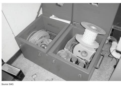
Figure 3: Type 3 (Portable Day-Box) Explosives Storage Magazine in Pennsylvania
