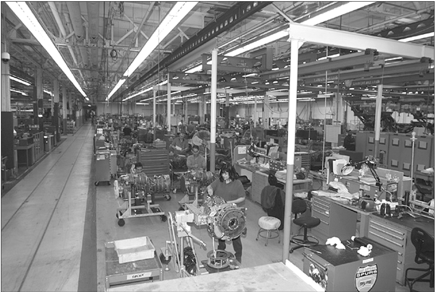
Figure 4: Corpus Christi T700 Engine Repair Line
