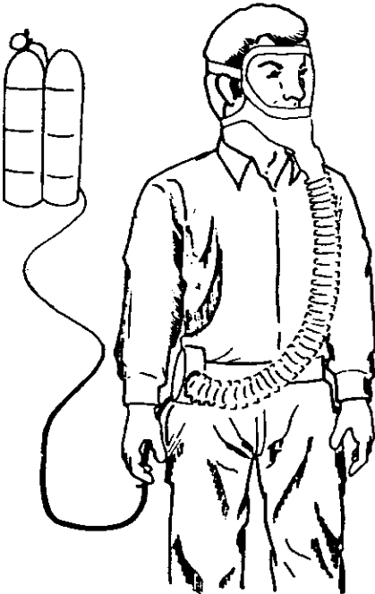
Supplied Air Respirator with Auxiliary, Escape-only SCBA
