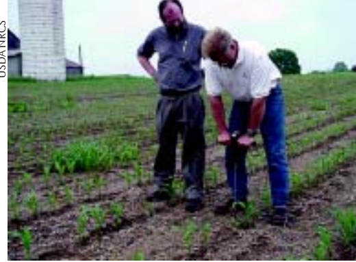
Bob Wade Jr. and Dan Towery, Conservation Technology Information Center, test for soil compaction in a field that has been no-tilled continuously for over 17 years.
