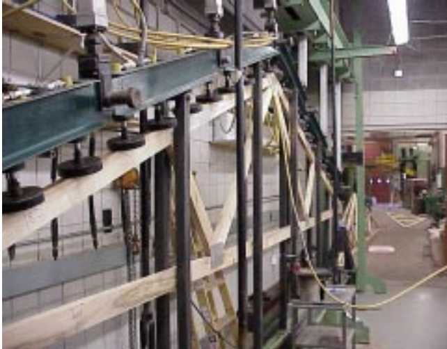
Test being conducted on full-size maple truss
