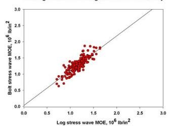
It is also possible to monitor the quality of growing trees as an indication of future wood quality. Studies indicate that direct monitoring of MOE may provide a better indicator of stiffness than does the traditional approach of monitoring specific gravity.
