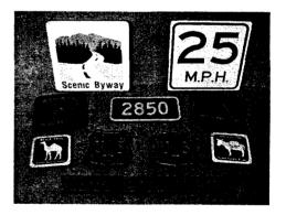
Figure 1. Examples of durable and stable outdoor sign made from compression-molded juniper-plastic composites using a 50/50% mixture of juniper fiber and recycled polypropylene.
