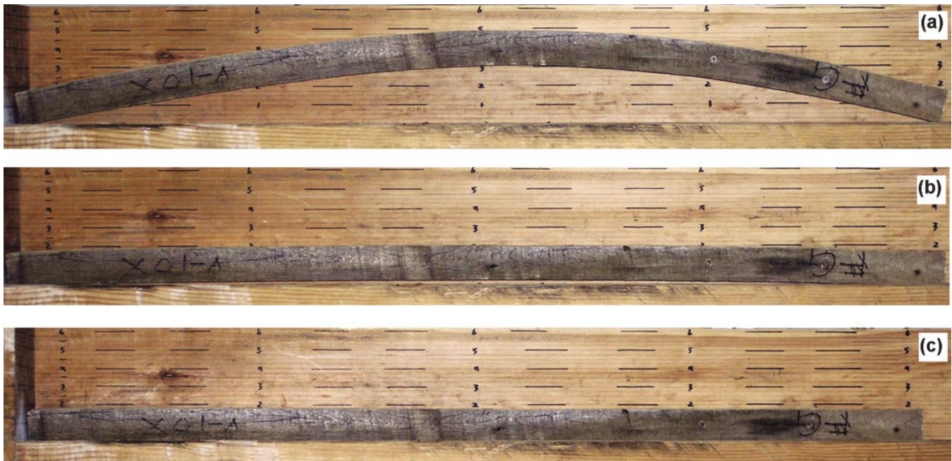
Figure 8—Effect of microwave heating and compressive pressing on bow of 1.2-m- (4-ft-) long board with approximately 10% initial bow: (a) before microwave pressing; (b) immediately after heating at 150°C (302°F), holding at 150°C (302°F) for 5 min, pressing with continued microwave heating for another 10 min, and cooling for 15 min in closed platen; (c) after 48 h exposure to 20°C (68°F), 25%–35% relative humidity environment.
