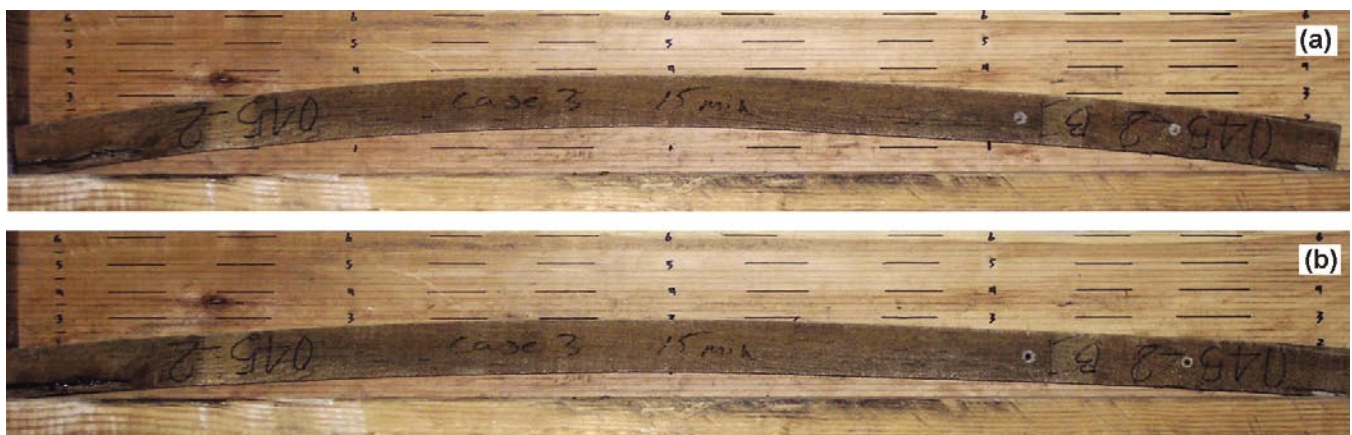
Figure 7—Effect of initial microwave heating to 140°C (284°F) in pressurized chamber and subsequent compressive pressing for 15 min on bow of 1.2-m- (4-ft-) long board with 7.5% initial bow: (a) before microwave heating; (b) immediately after removal from microwave chamber. Board showed approximately 50% reduction in bow.
