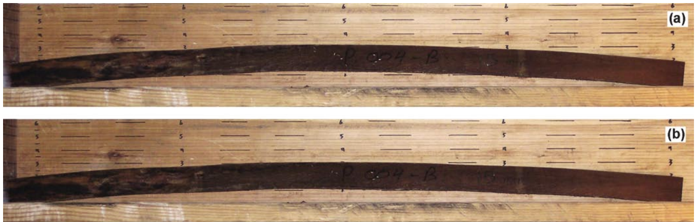
Figure 6—Effect of compressive pressing (15 min) without initial microwave heating on bow of 1.2-m- (4-ft-) long board with 6.5% initial bow: (a) before pressing; (b) immediately after removal from microwave chamber. Board showed virtually no reduction in bow.
