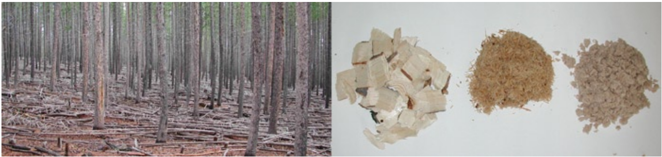
Figure 2—The process can produce 3DEF using recycled paper fiber or virgin timber or fire-prone forest residuals, such as shown on forest floor (left). When timber is used, it is chipped and then processed into various fiber types (right), depending on desired end-product properties.
