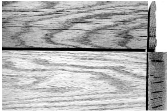
Figure 12-11. Board machined into millwork shows honeycomb (top). Surface of planed red oak board shows no honeycomb (bottom).
