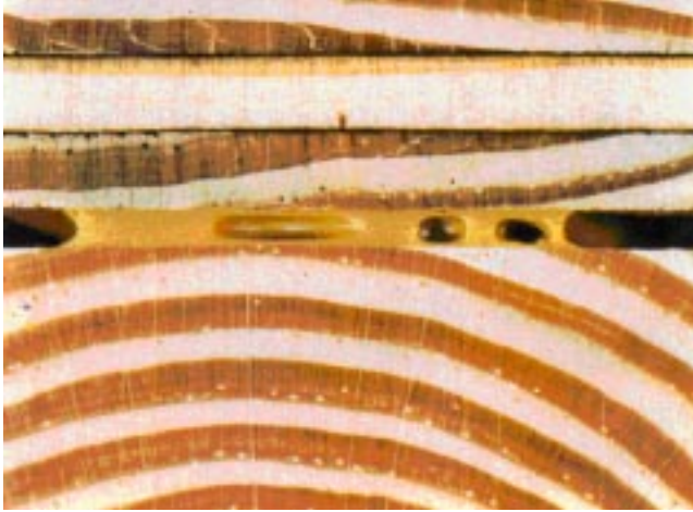
Figure 9–11. Gap-filling construction adhesive in field-assembled plywood floor system.
