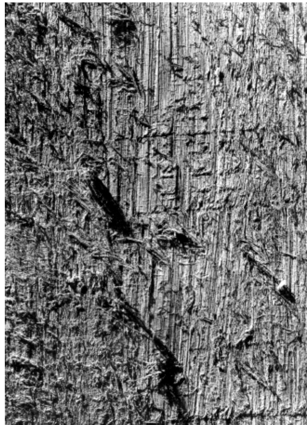
Figure 4-7. Projecting tension wood fibers on sawn surface of mahogany board.
