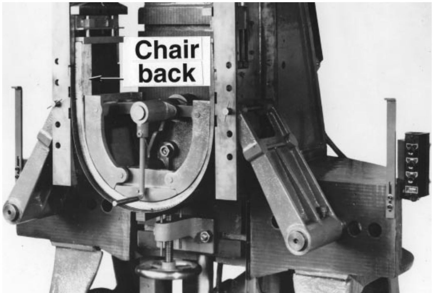
Figure 19-1. Chair back being bent through an arc of 180° in a bending machine.
