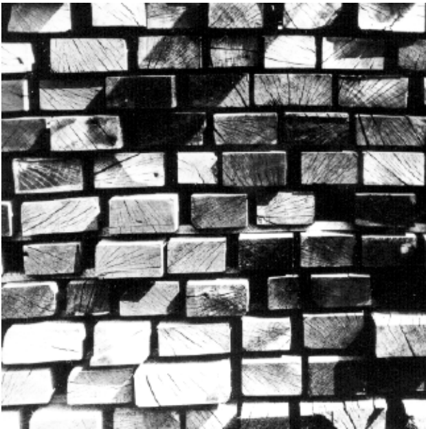
Figure 12-9. End checking in oak lumber.
