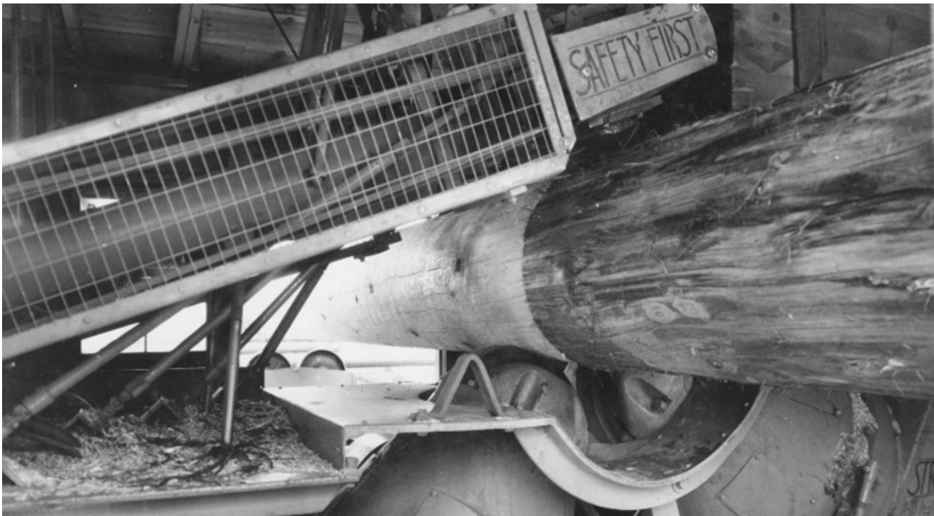
Figure 14-1. Machine peeling of poles. The outer bark has been removed by hand, and the inner bark is being peeled by machine. Frequently, all the bark is removed by machine.
