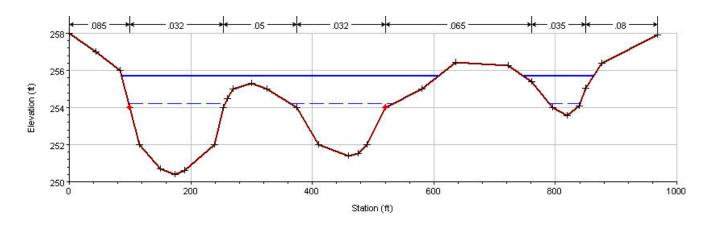
The three flow channels, with a Manning's n-value of near 0.032 are much more efficient at passing discharge than was assumed by the modeler who allowed everthing right of the first channel to be represented by a 0.05 roughness value.
