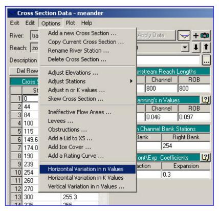
"Horizontal Variation in n Values" is one of the options toward the bottom of the list. When selected, the station / elevation table is given a third column, as shown at right, for specifying additional roughness values which are given between any two cross-section points. More appropriate roughnesses have been entered into the table.
