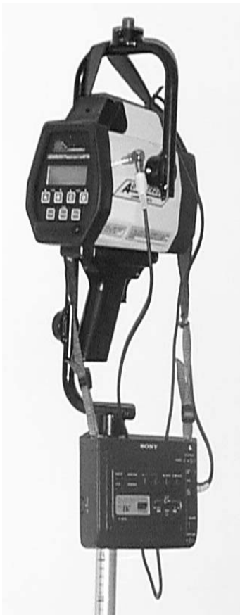
Figure 1—Camera rangefinder prototype used in this study.
