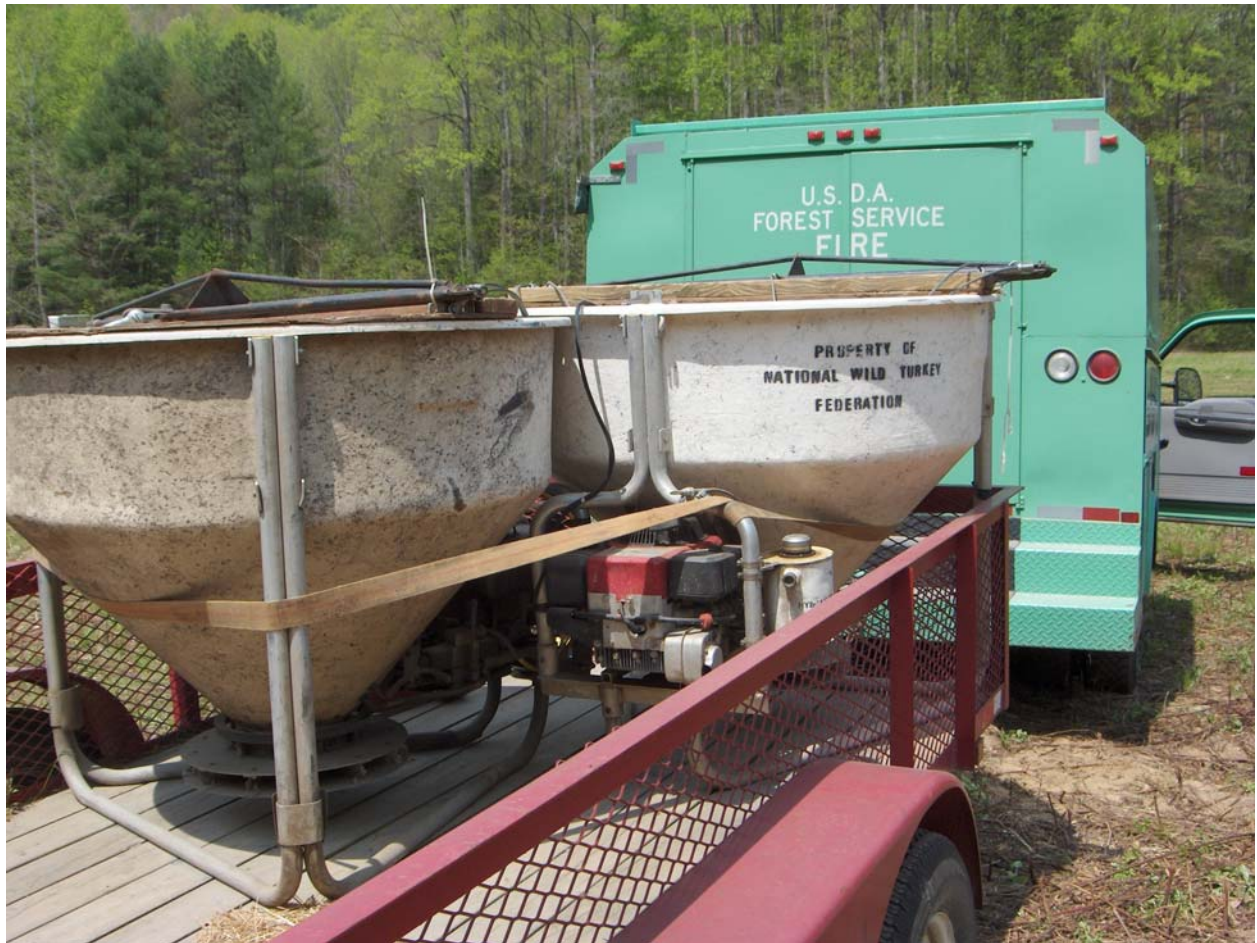
Seed Mixing Buckets Used in Aerial Seeding of Landslides on Grandfather District
