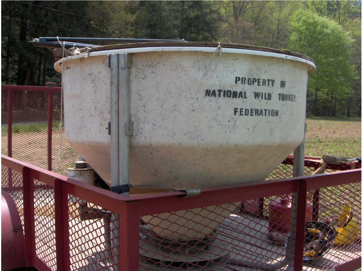
Seed Mixing Bucket to be Attached to Helicopter
