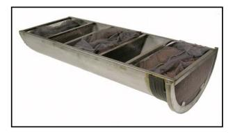
Another filtration unit is fabricated from stainless steel sheet metal. Loblolly pine bark particles (i.e., the absorption filter) are contained in fiberglass netting inside compartments of the unit. This unit is currently being tested for removal of phosphorus in drainage from cranberry bogs.
