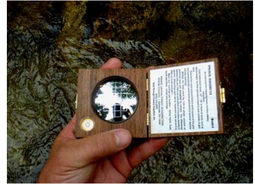
A spherical densiometer provides an estimate of a stream's overstory vegetation density. The measurement is stated as an average of four readings facing north, south, east and west. This estimate is a measurement of "canopy cover".
