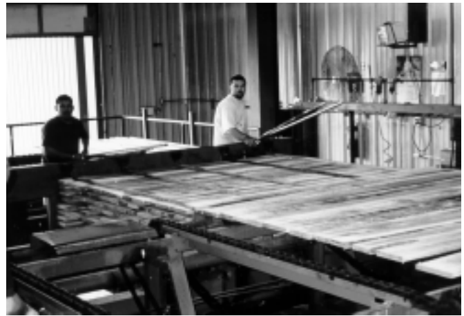
Figure 3.2—Stacking of stickered package of lumber.
