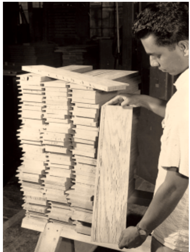
Figure 9.1—Extensive surface checking in oak lumber.
