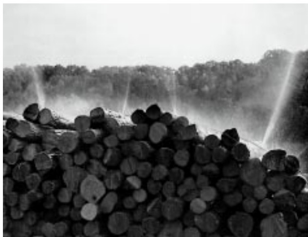
Figure 3.1—Water spraying equipment can often be used effectively on decked logs to prevent deterioration over short periods.
