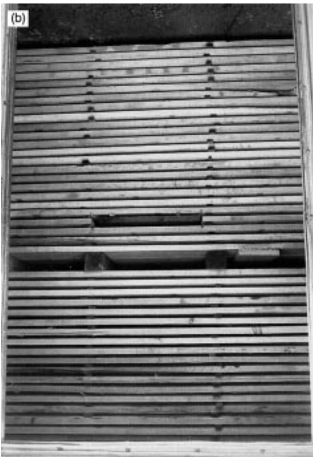
Figure 7.5—Placement of kiln samples in pockets. (a) Schematic of kiln samples placed in pockets built in the side of a load of lumber. Pockets should be deep enough so that the kiln samples do not project beyond the edge of the load. (b) Photograph of kiln sample in place.
