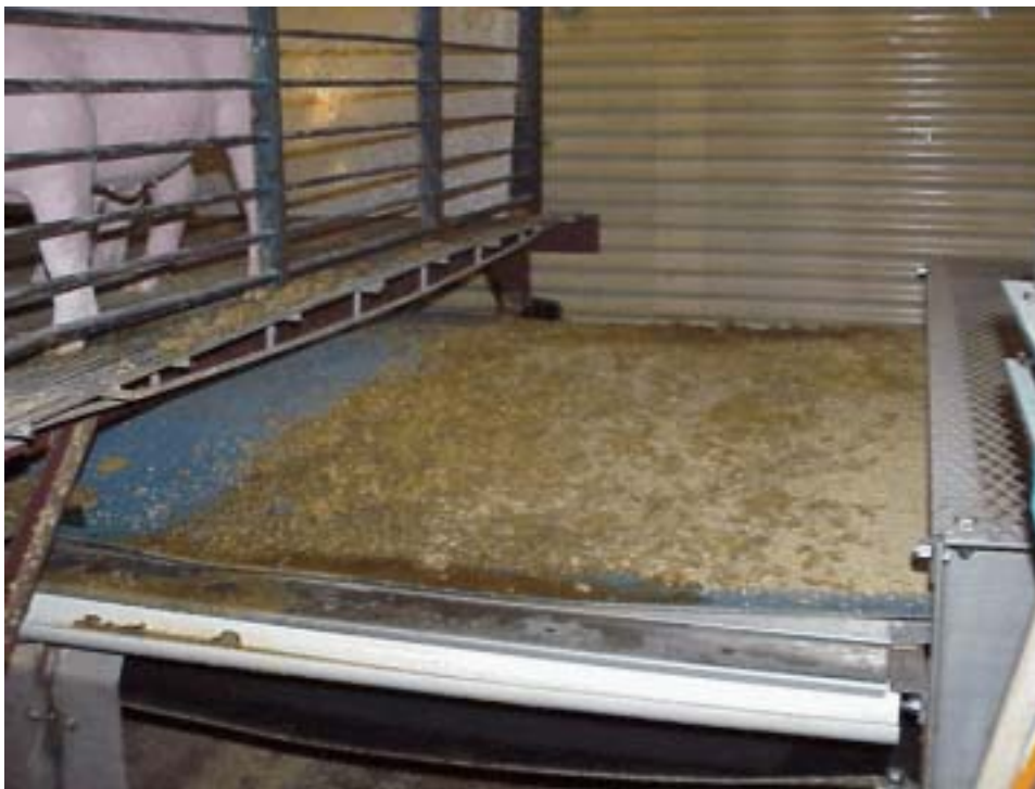
Figure 1. Belt system during solids removal
