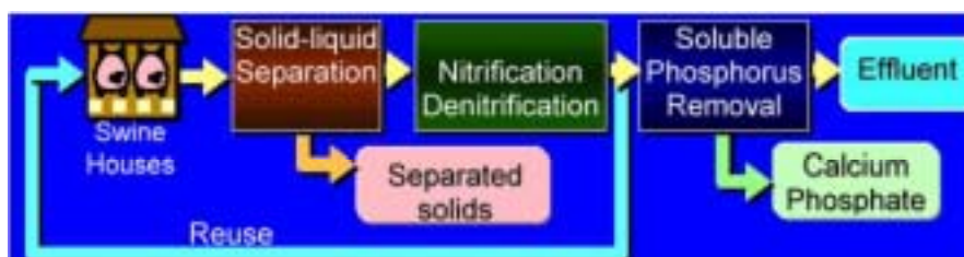
Figure 3 . Process treatment in Goshen Facility (USA).
