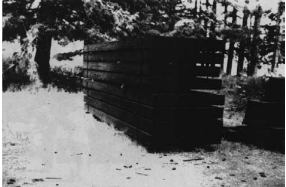
Figure 12-9. - Glulam deck panels stacked for storage.
