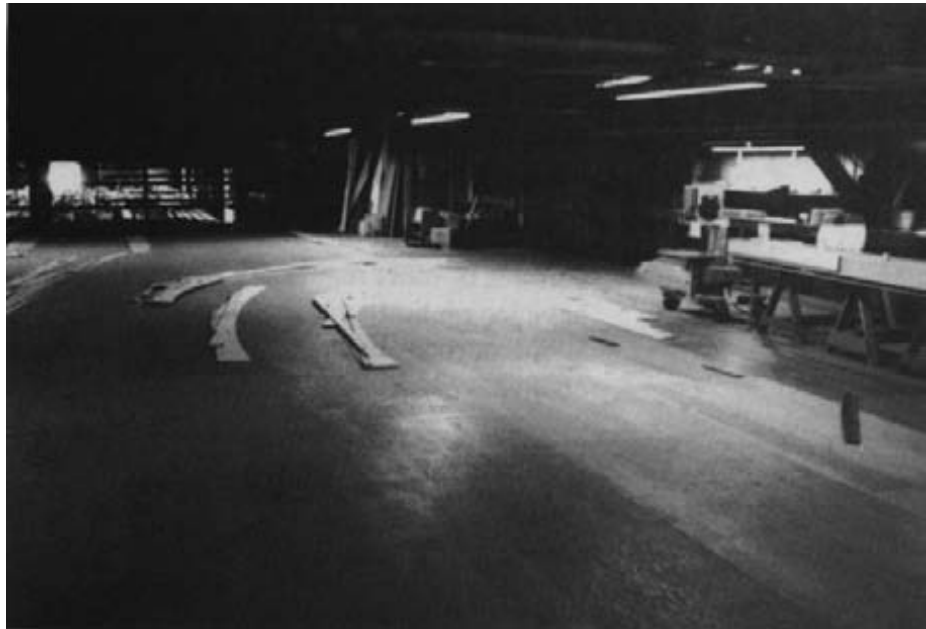
Figure 12-3. - Template production area at a glulam manufacturing plant. Plywood templates shown in the background are used to ensure consistent, accurate, and complete fabrication of multiple glulam members.
