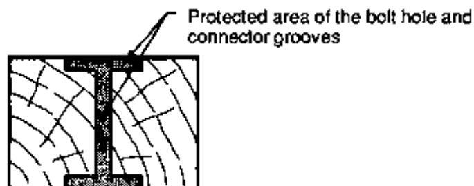
Figure 5-28. - The net area at a timber connector is equal to the gross area of the member minus the projected area of the bolt hole and connector grooves.
