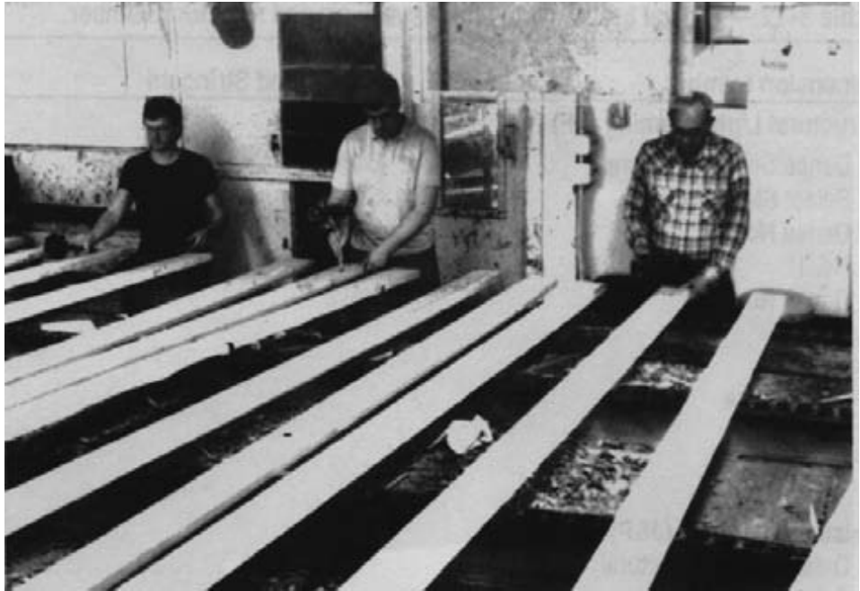
Figure 3-26.- Sawn lumber being visually graded and marked at a sawmill (photo courtesy of Funk Lumber Co.).
