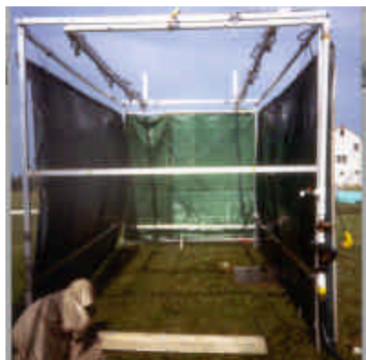
Rainfall simulator used during the development of the P Index
