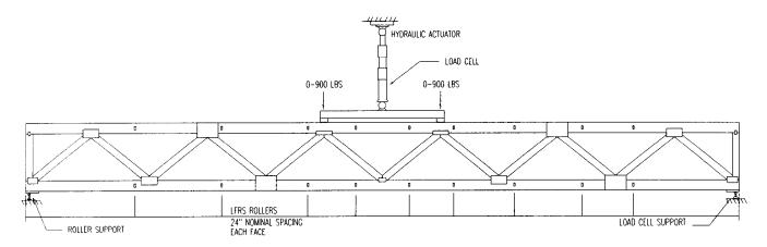
Figure 1 -Configuration of Truss Fatigue Test
