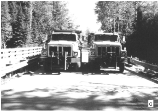
Figure 17—Load cases 1, 2, and 3 used during load testing of span 1 (west): (a) load case 1, (b) load case 2, (c) load case 3.
