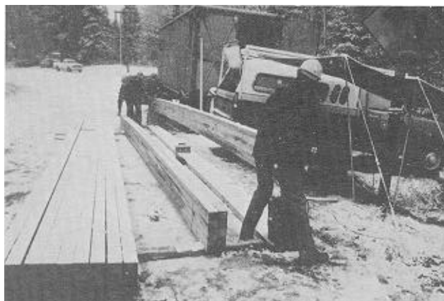
Figure 10—Measurement of the beam lamination MOE at the bridge construction site using the transverse vibration technique. (M92 0009-7)
