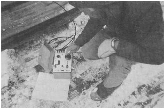
Figure 12—Reading a load cell with a portable strain indicator. (M92 0001-27A)
