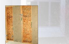
MOISTURE RESEARCH: Forest Products Laboratory (FPL) is working in cooperation with Syracuse University to measure air pressure, temperature, and relative humidity in the wall cavities. The cellulose insulation is being replaced with fiberglass to match the controlled conditions of the Syracuse lab. The study includes state-of-the-art instrumentation engineered by FPL researchers to supply actual field measurements of moisture and airflow in the wall cavities.
