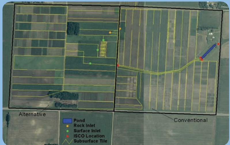
Alternative (65 ha) and conventional (65 ha) management areas, including surface and subsurface drainage systems in southwest Minnesota
