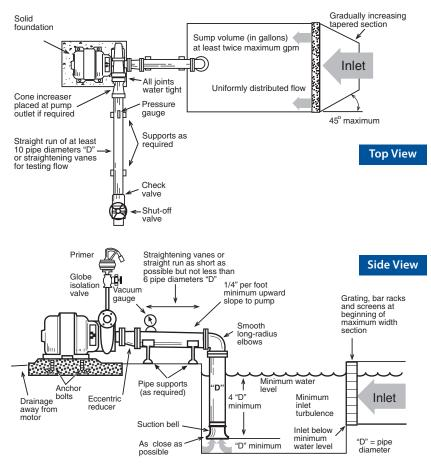
(Adapted from Energy Efficient Pumping Standards, Utah Power & Light Company.)
