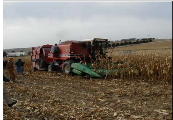
Figure 3. One-pass harvester for corn grain and stover. G.R. Quick, Iowa State University
