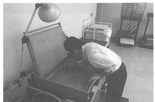
Similar to traditional Japanese paper making techniques, this leaf-casting machine is highly valued in restoration work. With this process the fibers of washi paper fill in the damaged parts of documents.
