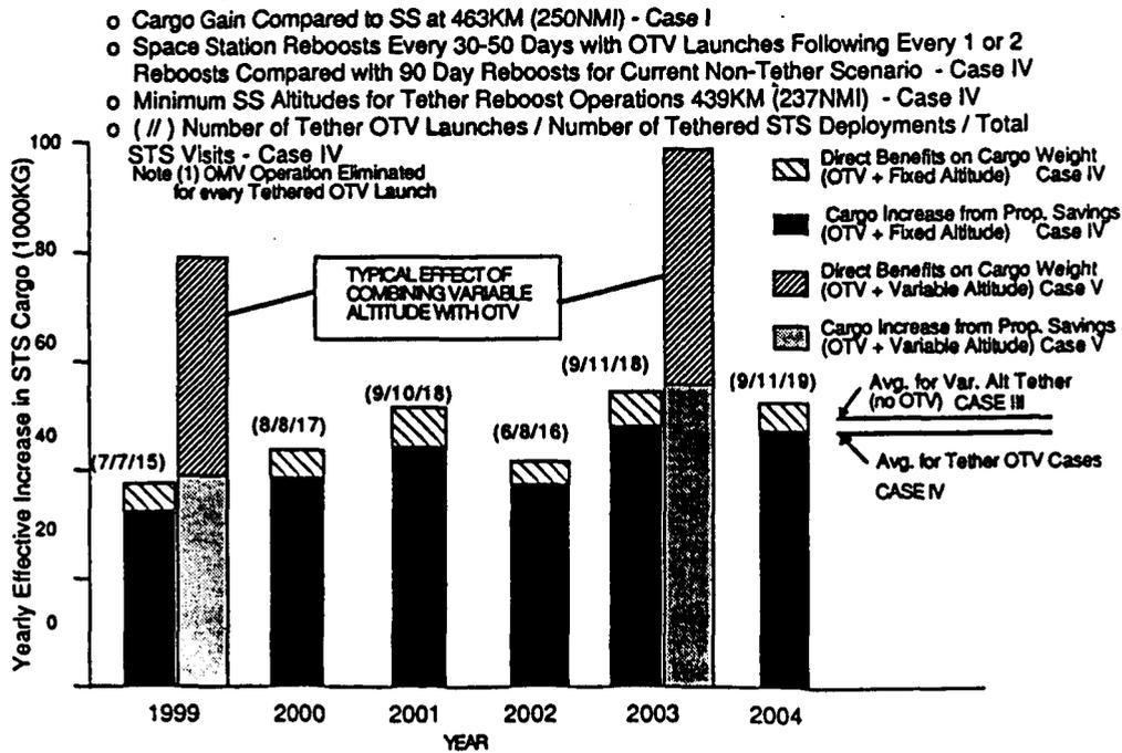
Fig. 7 - Benefit of Combining Tethered OTV and Shuttle Operations on the Space Station
