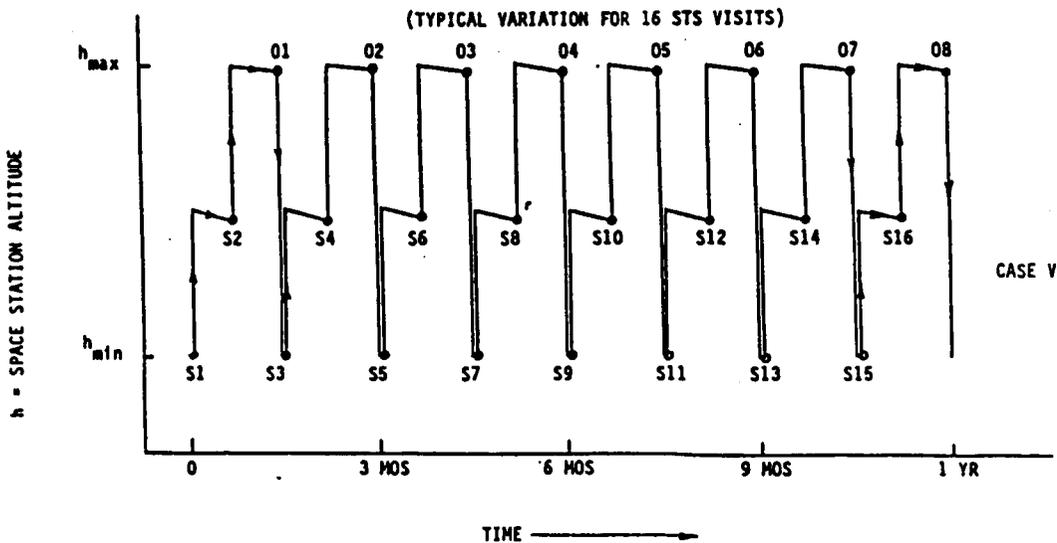
Fig. 5 Momentum Balance - Tethered OTV/STS at Variable Altitude
