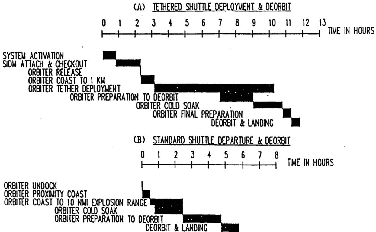
Fig. 9 Tethered and Standard Shuttle Deorbit Timelines
