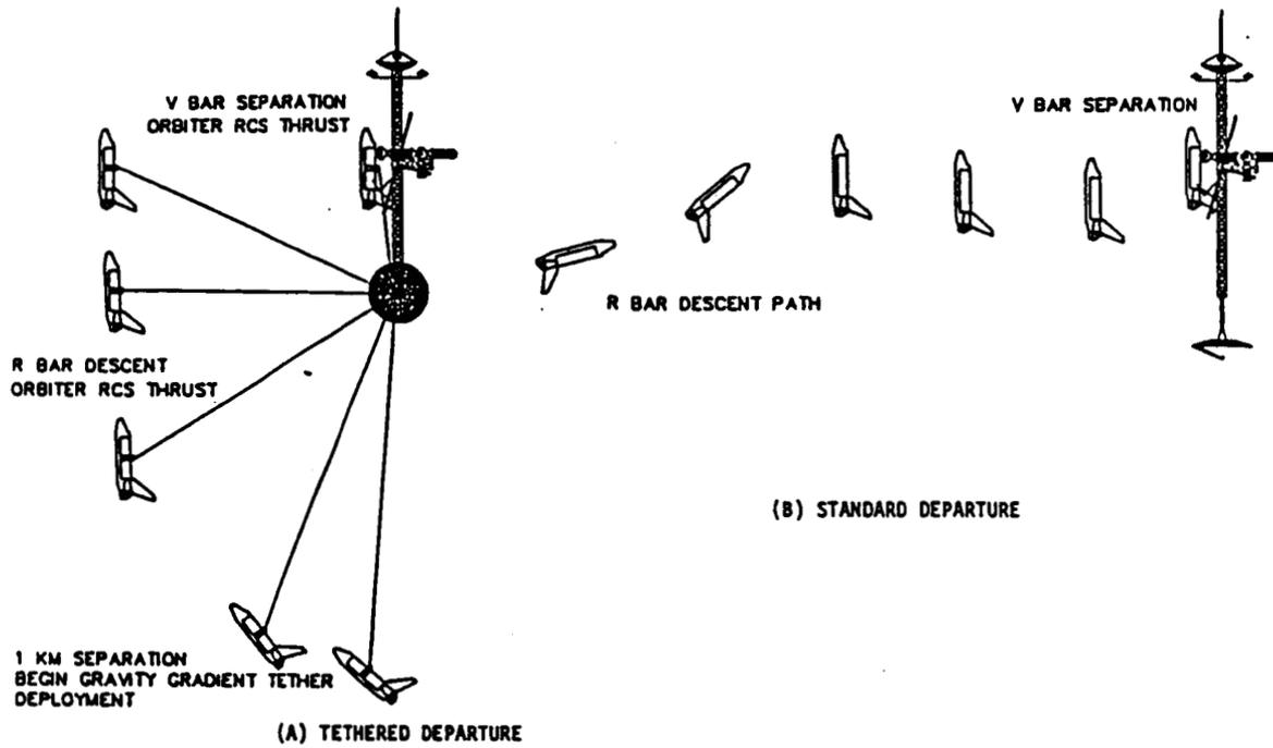
Fig. 8 Tethered and Standard Departure of Shuttle from Space Station
