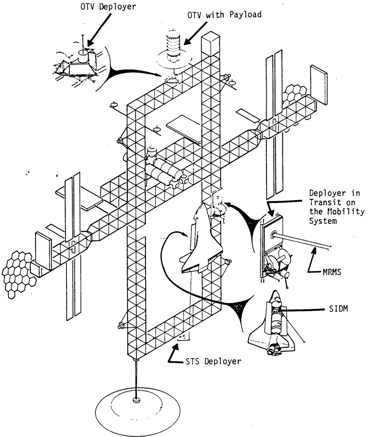
Fig. 1 Space Station with Deployer System
