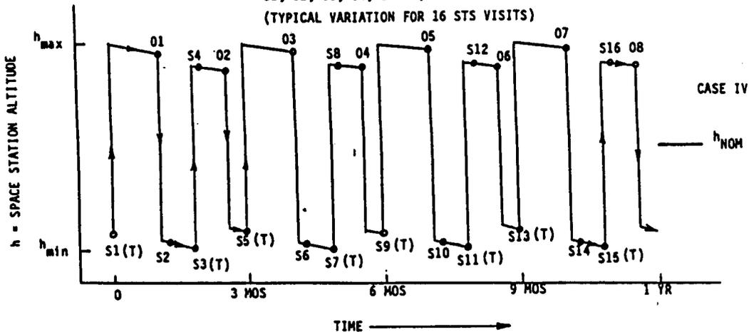
Fig. 4 Momentum Balance - Tethered OTV/STS at Current Altitude
