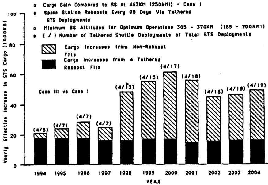
Fig. 6 - Benefit of Variable Altitude Operations - Tethered Satellite
