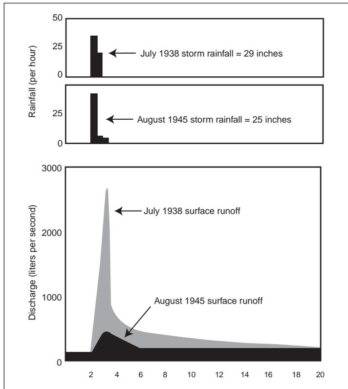
Figure 18—Rainfall and runoff hydrographs for the White Hollow, Tennessee, watershed before and after watershed rehabilitation (from Smallshaw and Ackerman 1951).
