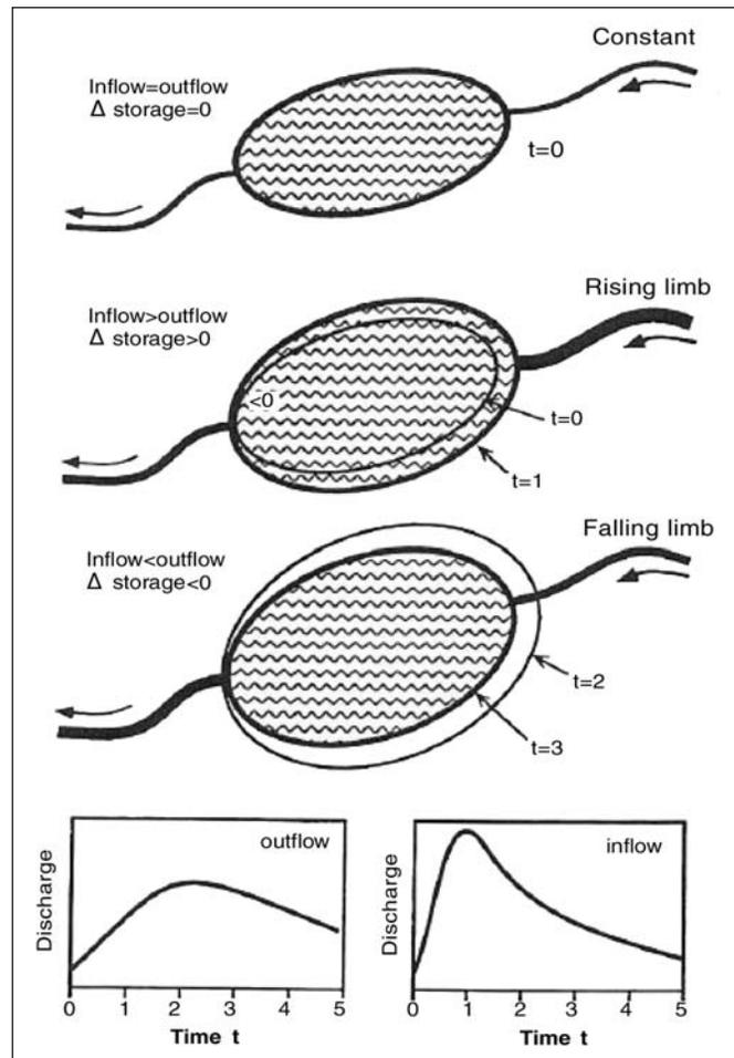
Figure 12—Flood routing in a channel with a reservoir during constant flow ( $t = 0$ ) and the rising ( $t = 1$ ) and falling ( $t = 3$ ) limbs of a peak flow event. Volumes of storage in the reservoir during three time periods are represented by oval size; finer lines outline the water surface area in the reservoir during the preceding time interval. The patterned oval depicts reservoir level at corresponding inflow and outflow rates (from Ziemer and Lisle 1998).
