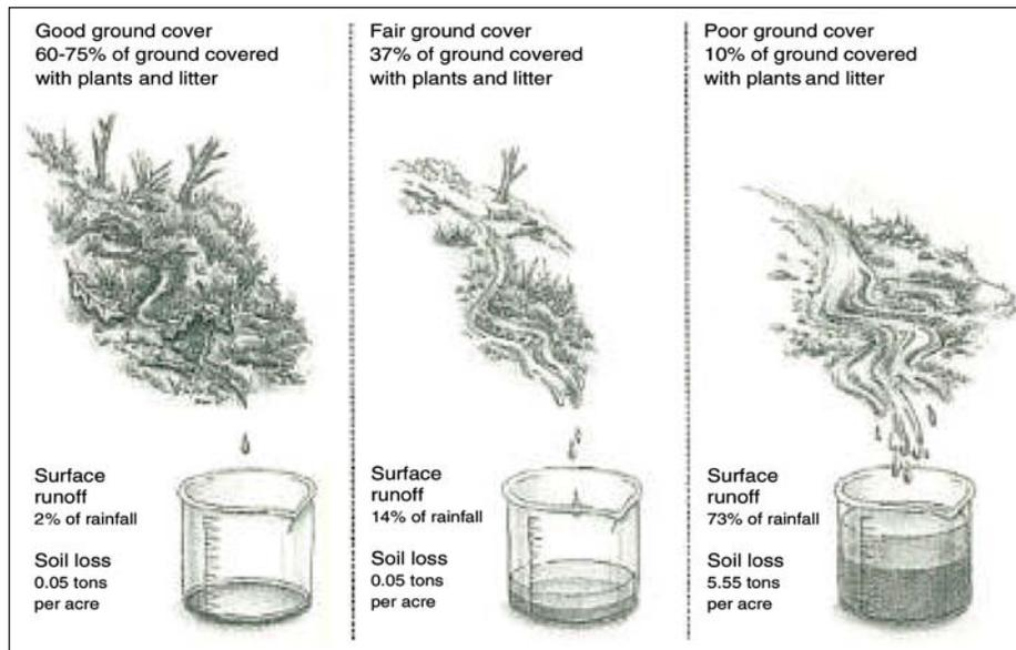
Figure 17—Experimental results of the effects of watershed condition on rainstorm runoff and erosion (from Sedell et al. 2000).
