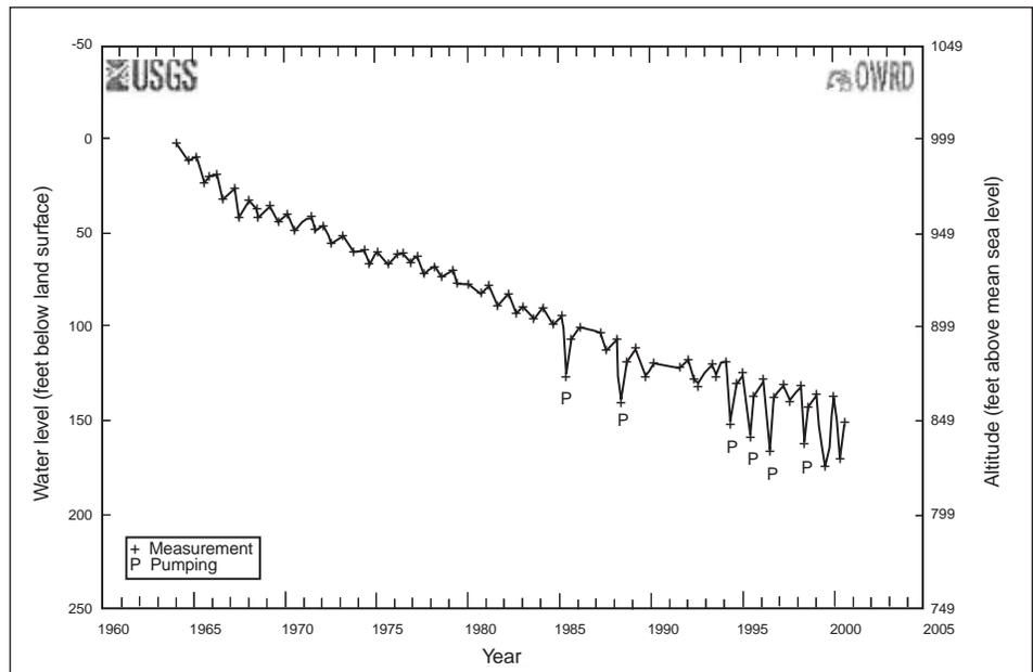
Figure 16—Water-level decline in Well 502 in Linn County, Oregon. Water level has declined 150 feet in 30 years owing to pumping of groundwater (from Orzol et al. 2000).
