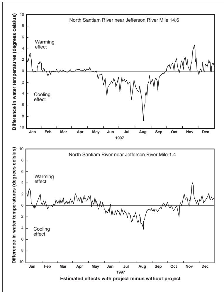
Figure 20—Simulated water temperatures with, and without, U.S. Army Corps of Engineers' reservoirs at selected sites on the North and South Santiam Rivers, 1977 (Hansen and Crumrine 1991).
