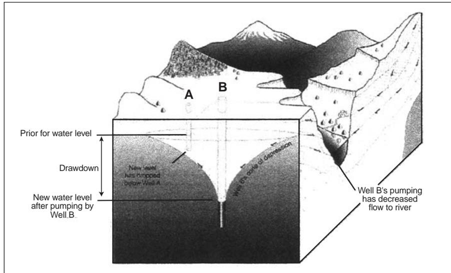
Figure 15—Groundwater dynamics around major wells. As groundwater is pumped, the cone around wells such as B expands, intercepting water bound for streams (from Bastasch 1998).
