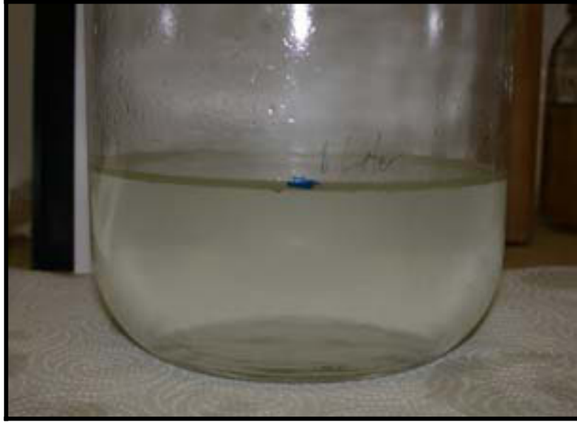
Figure 1. Stage 2 microcosm bottom-water. 200 mL pooled bottom-water from Stage 1, Round 2 microcosms have been added to 800 mL SBW.
