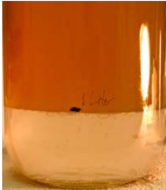
Figure 2. Stage 2 microcosm just after set-up: NALSD over SBW depicted in figure 1.
