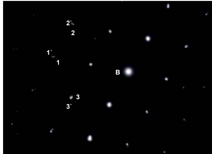
Figure 4-21. SADP near the interface between CIS film and GaAs substrate, W560.
