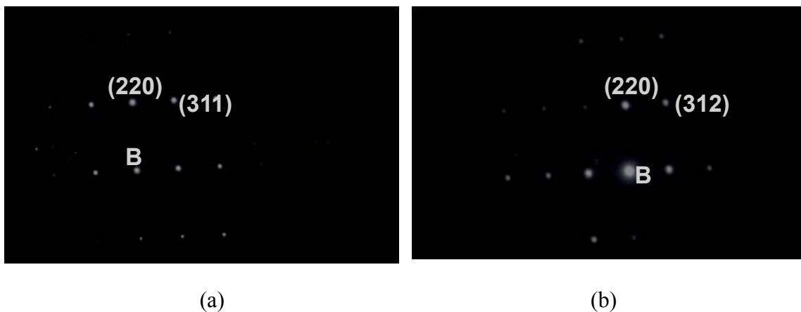
Figure 4-28. SAD pattern of island region of the Cu-rich, Na-dosed sample (W584) at [-1\ 1\ 2] zone axis: (a) upper layer of island region ( \text{Cu}_{1.5}\text{Se} ), (b) lower area of the island region (CIS).
