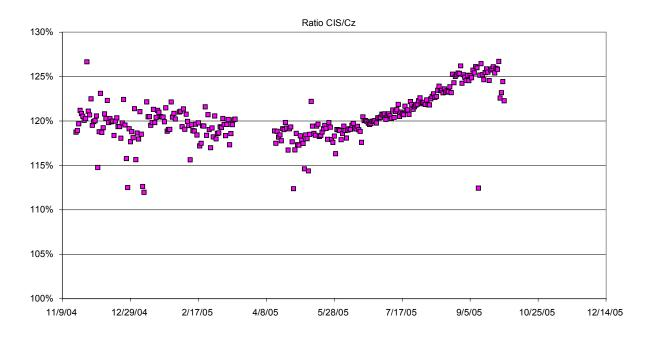
Figure 53. The ratio of the energy produced by a CIS array compared to a silicon array in a sideby-side test on the roof of the R&D building in Camarillo.
