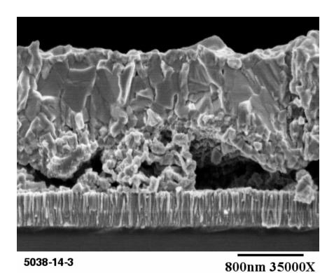
Figure 25. SEM image of pre sputter dose baseline absorber with lower than normal Na.
