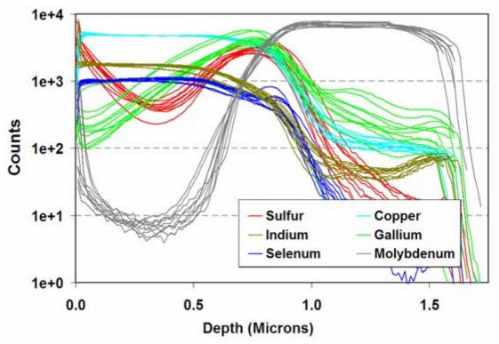
Figure 27. SIMS molecular scan color-coded by element.
