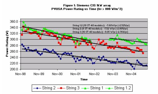
Figure 47. Outdoor measurements of the third CIS array delivered to NREL. Power losses of 2.5 to 2.8 percent per year were observed.
