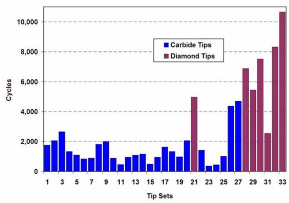
Figure 38. Lifetime comparison of carbide and diamond tips for mechanical scribing.
