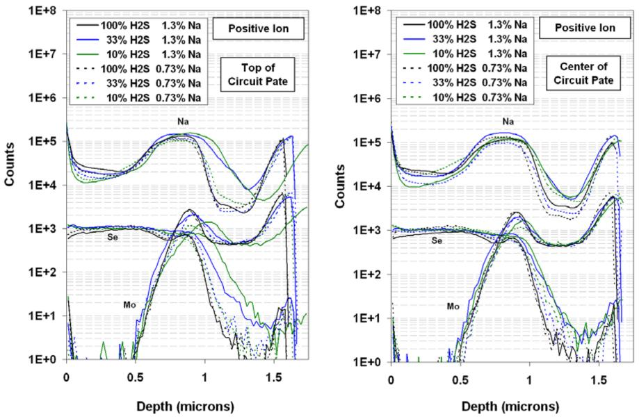
Figure 21. Positive ion SIMS profiles - top and center, emphasizing Na.
