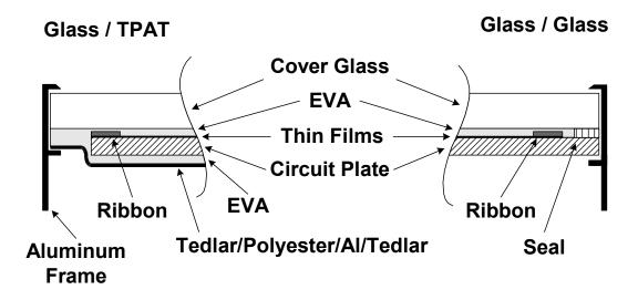
Figure 8. "TPAT" backsheet and "glass/glass" package designs.
