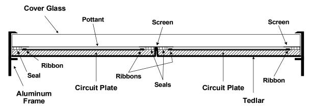
Figure 10. Eclipse 80-C glass/glass package.
