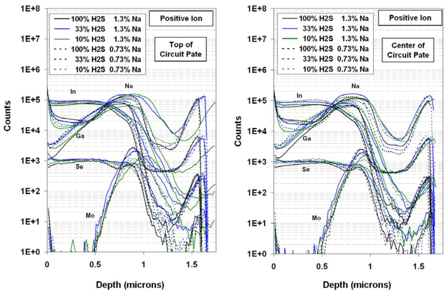
Figure 20. Positive ion SIMS profiles - top and center, all elements.
