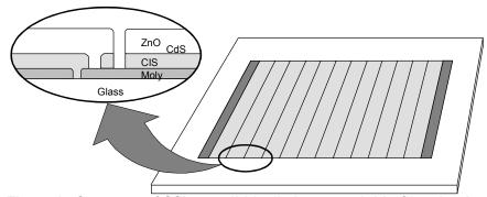
Figure 1. Structure of SSI monolithically integrated thin-film circuits.
