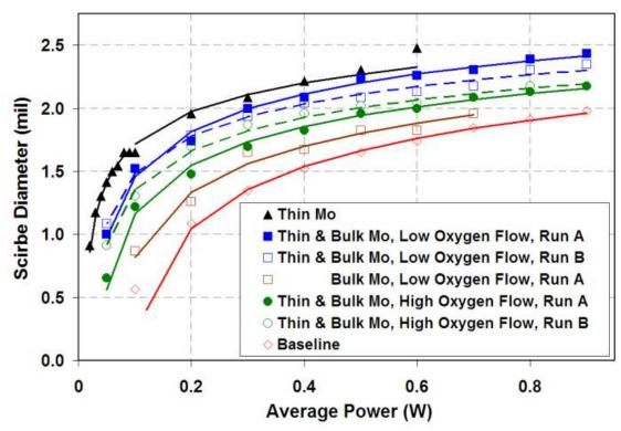
Figure 36. P1 scribe diamater vs. Mo process and P1 power
