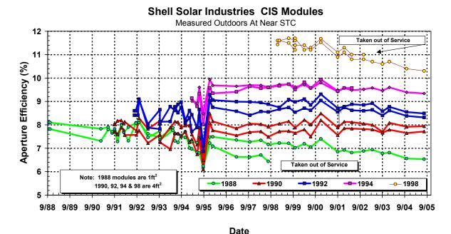
Figure 46. Efficiency measured using outdoors on CIS modules deployed at NREL.
