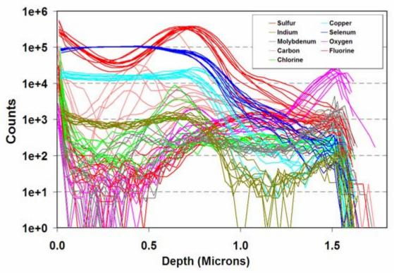
Figure 33. SIMS negative ion scan color-coded by element.
