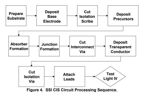
This process starts with ordinary sodalime window glass. An SiO<sub>2</sub> barrier layer is deposited to minimize sodium diffusion from the substrate and thereby improve adhesion between the CIS
