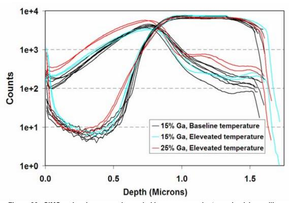
Figure 30. SIMS molecular scan color-coded by process variant, emphasizing gallium
