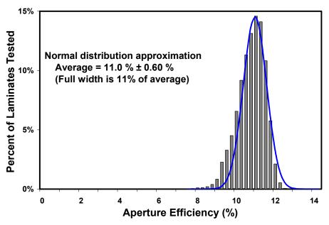
Figure 13. Production distribution for 1x4-ft. laminates produced during 2003.
