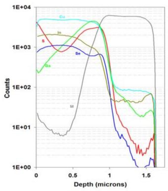
Figure 6. Typical elemental profile for the SSI graded absorber (SIMS from NREL).
