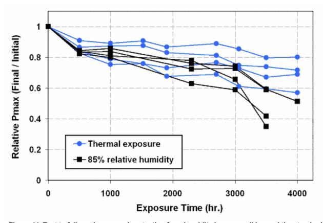
Figure 44. Test to failure shows good protection from humidity ingress well beyond the standard 1000-hour accelerated test.
