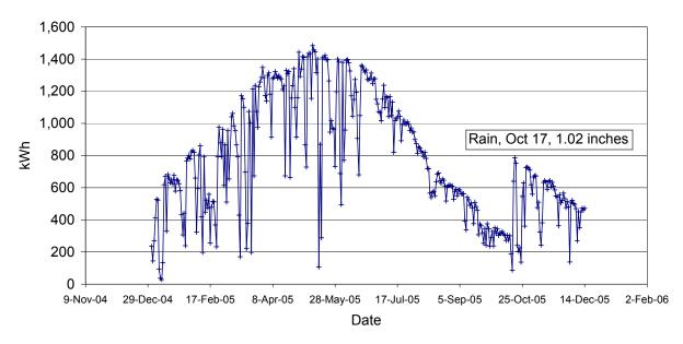
Figure 49. Daily energy production from the 245-kW rooftop array. It rained 1.02 inches of water on October 17, 2005, resulting in a dramatic increase in production.
