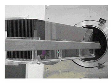
Figure 5. Photograph of 1x4-ft circuits in front of absorber formation reactor.
