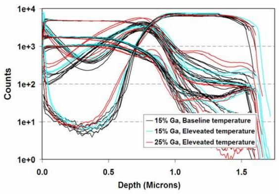
Figure 28. SIMS molecular scan color-coded by process variant.
