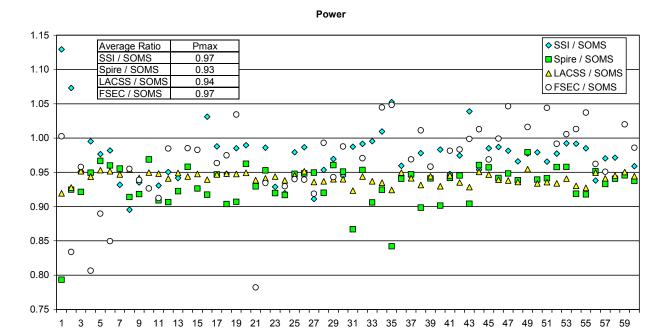
Figure 42. The ratio of the Power measured on the SSI LAPSS, the NREL Spire, the NREL LACSS and the FSEC Daystar are compared to the Power measured on the NREL SOMS.
