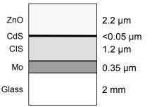
Figure 2. SSI CIS cell structure (not to scale).
