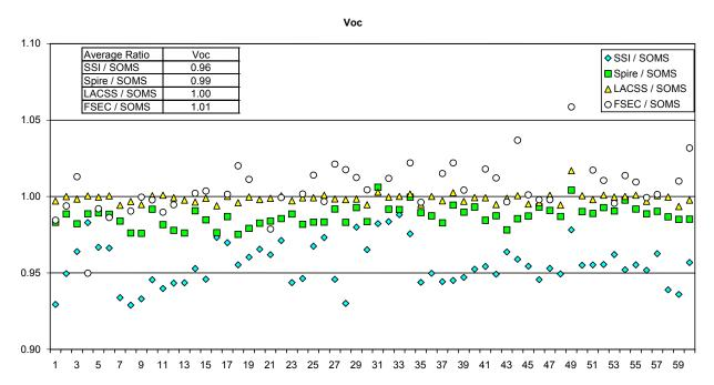
Figure 39. The ratio of the Voc measured on the SSI LAPSS, the NREL Spire, the NREL LACSS and the FSEC Daystar are compared to the Voc measured on the NREL SOMS.
