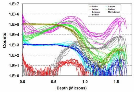
Figure 31. SIMS positive ion scan color-coded by element.
