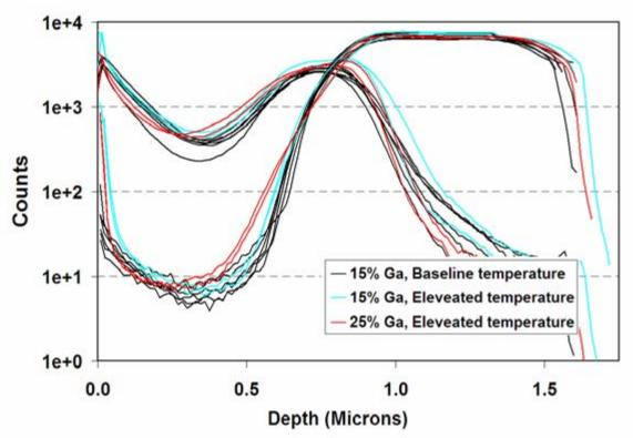
Figure 29. SIMS molecular scan color-coded by process variant, emphasizing sulfur.
