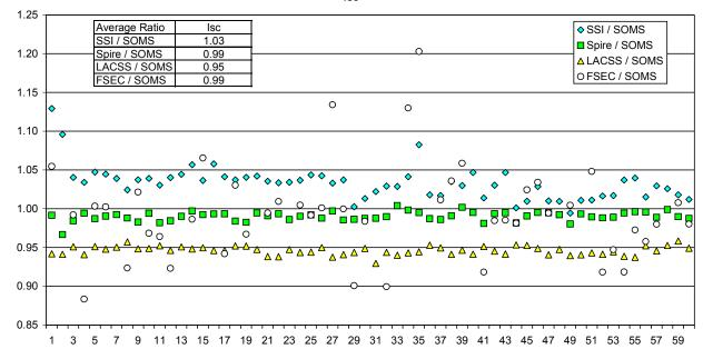
Figure 40. The ratio of the lsc measured on the SSI LAPSS, the NREL Spire, the NREL LACSS and the FSEC Daystar are compared to the lsc measured on the NREL SOMS.
