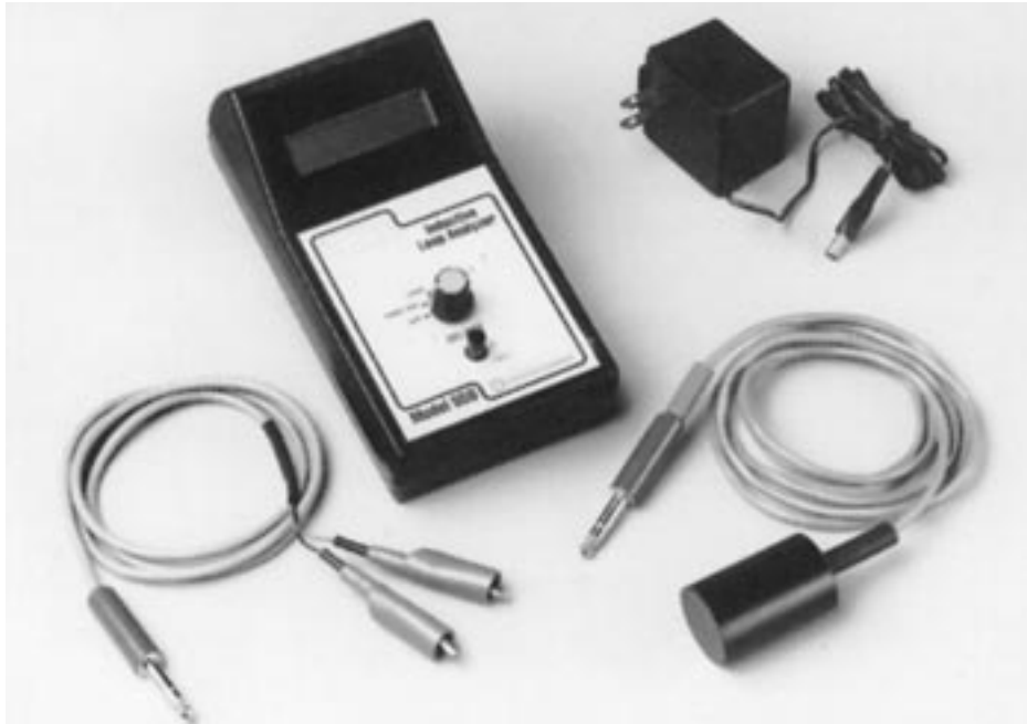
Figure 6-2. Model ILA-550 inductive-loop system analyzer. Measures the leakage resistance of a loop to ground at 500 V dc; frequency and relative signal strength of a loop network; loop inductance, resistance, and Q ; and change in inductance caused by vehicle driving over a loop (Photo courtesy of US Traffic Corp., Santa Fe Springs, CA).
