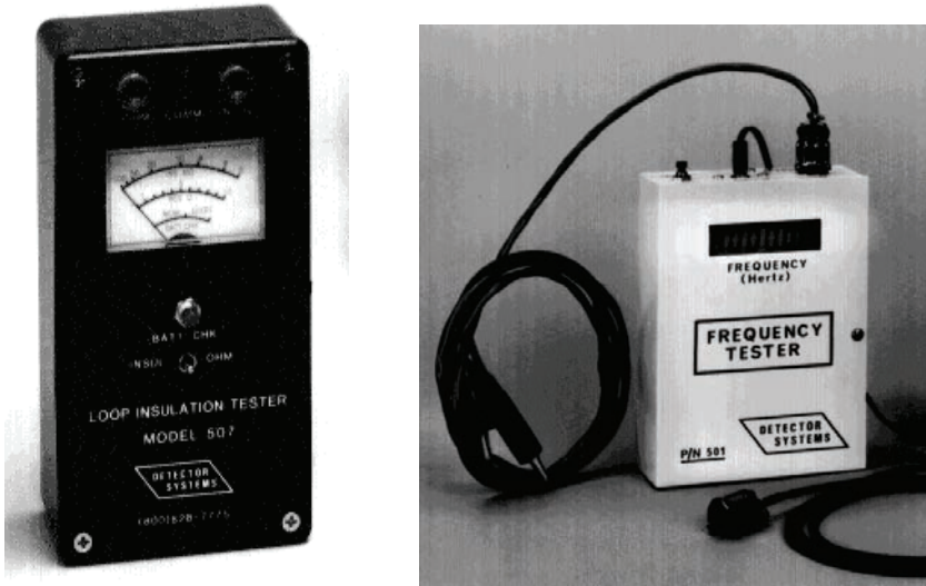
Figure 5-26. Loop test devices.
