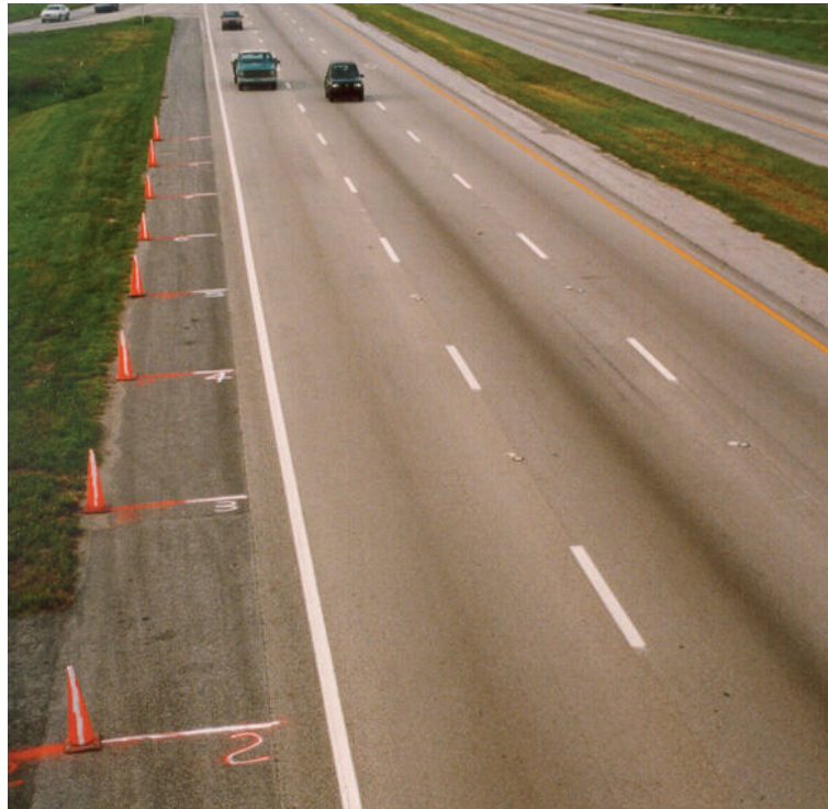
Figure 5-58. Up-lane distance measure aided by traffic cones placed at 25-ft (7.6-m) intervals (temporary markings).
