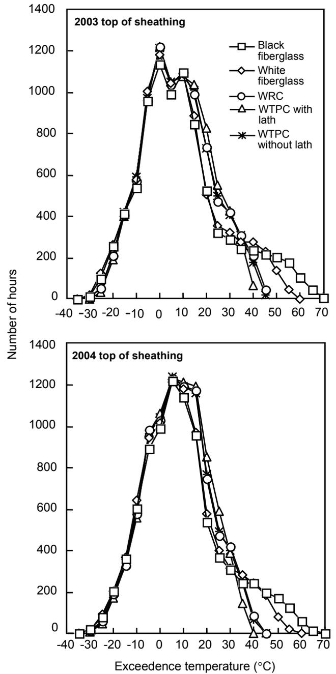
**Figure 5—Cumulative temperature histories at top surface of roof sheathing under various types of shingles.**
