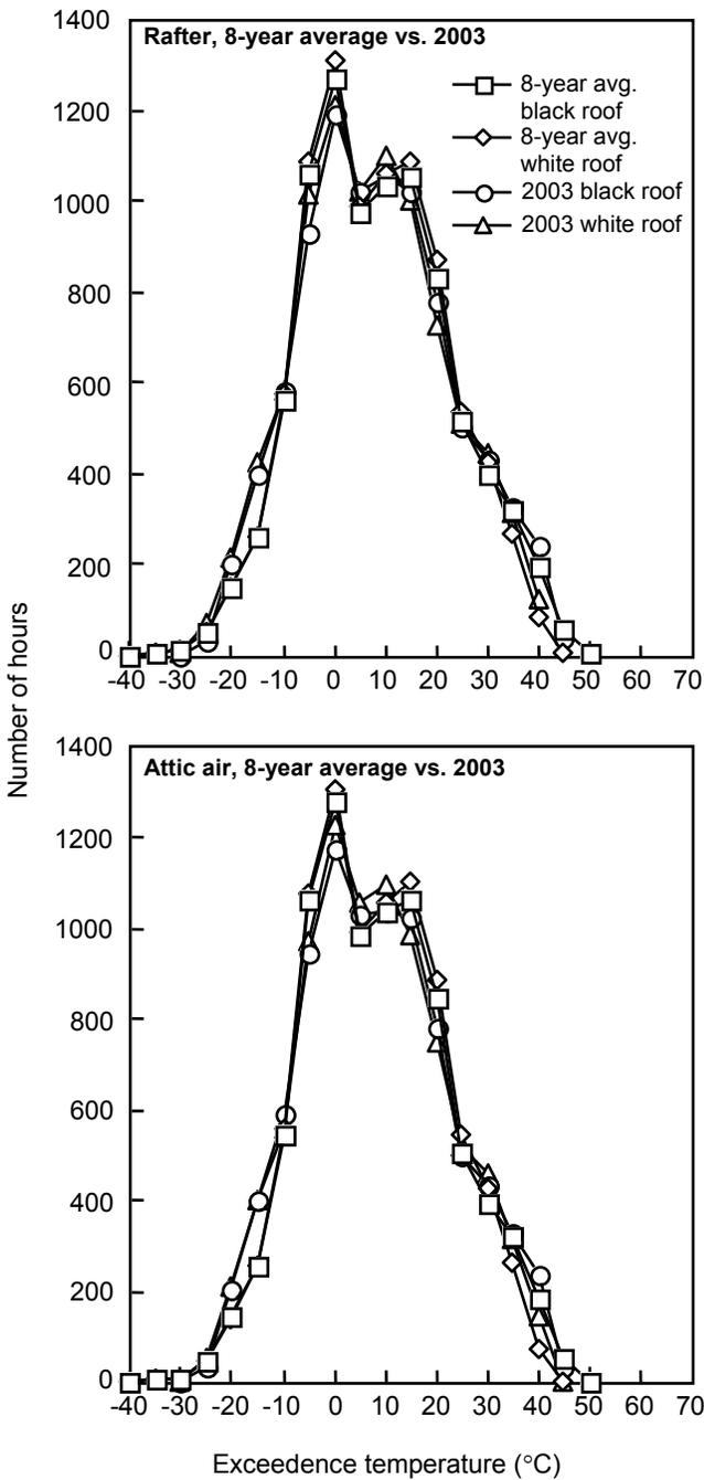
**Figure 10—Cumulative temperature histories of rafters and attic air in structures with black and white fiberglass shingles exposed from January to December 2003 compared to 8-year annualized data.**
