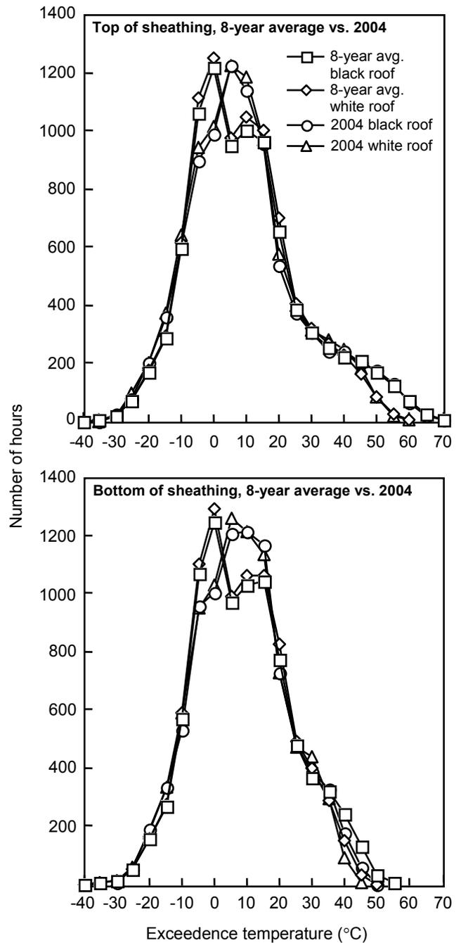
**Figure 11—Cumulative temperature histories at top and bottom of sheathing in structures with black and white fiberglass shingles exposed from January to December 2004 compared to 8-year annualized data.**
