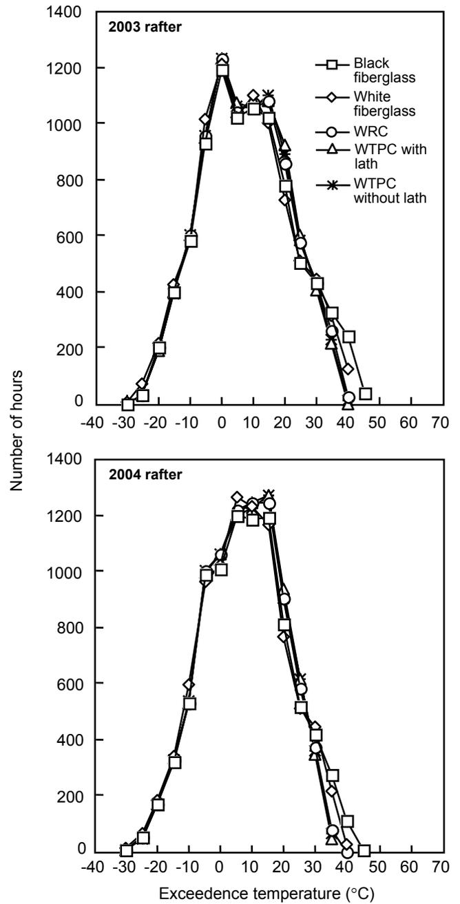
Figure 7—Cumulative temperature histories of interior core of roof rafters supporting sheathing under various types of shingles.
