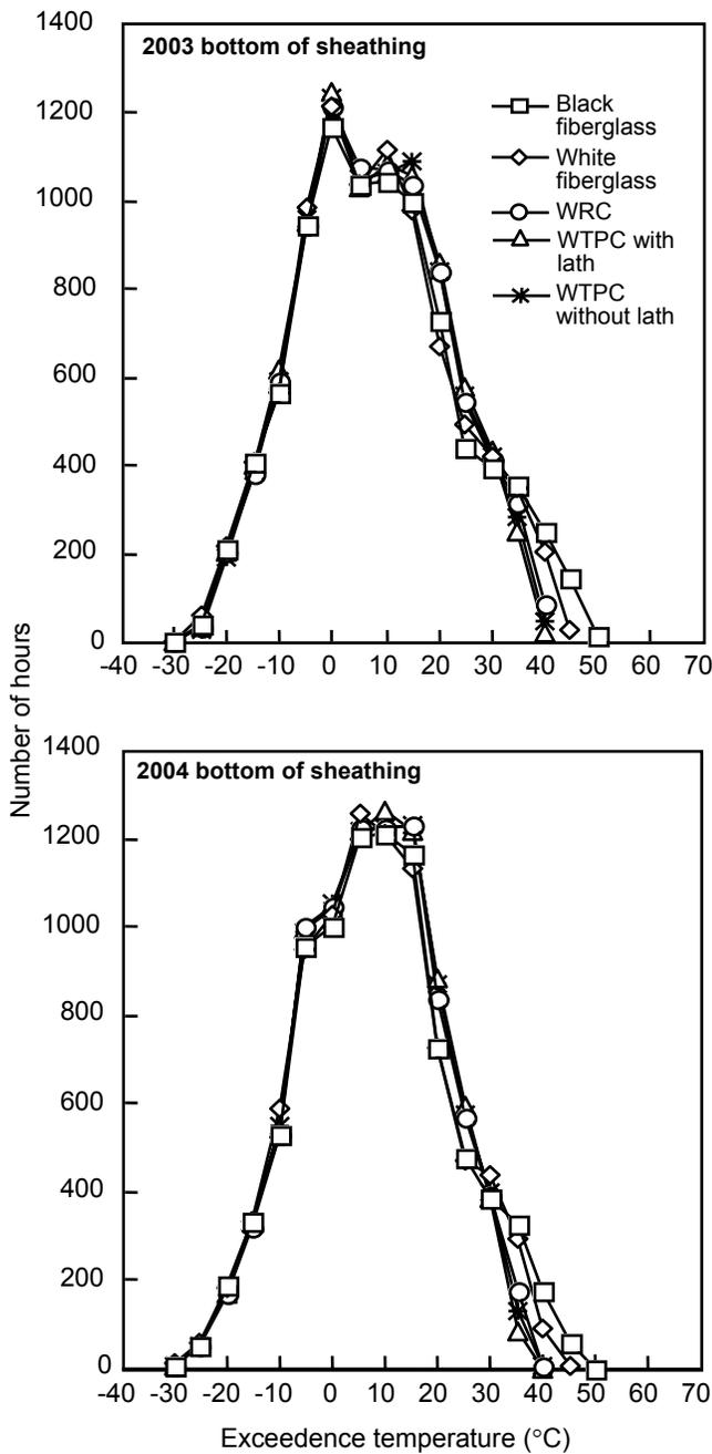
Figure 6—Cumulative temperature histories at bottom surface of roof sheathing under various types of shingles.
