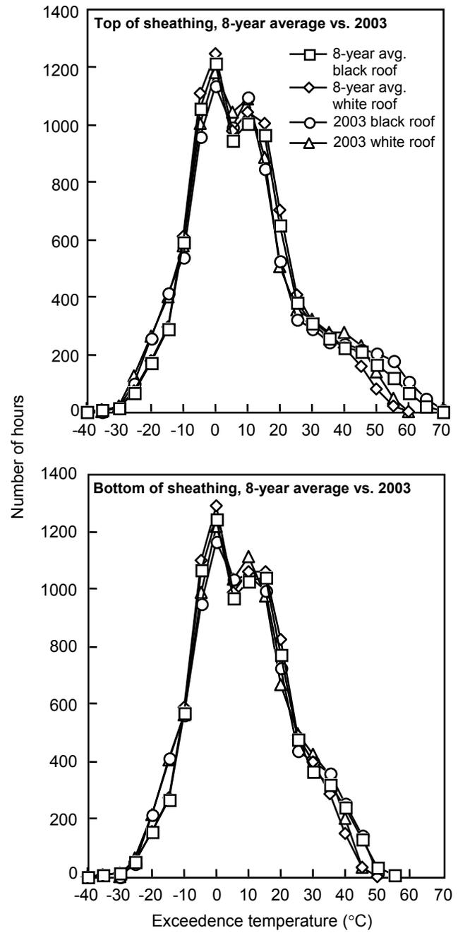
**Figure 9—Cumulative temperature histories at top and bottom of sheathing in structures with black and white fiberglass shingles exposed from January to December 2003 compared to 8-year (1992–1999) annualized data (Winandy and others 2000).**
