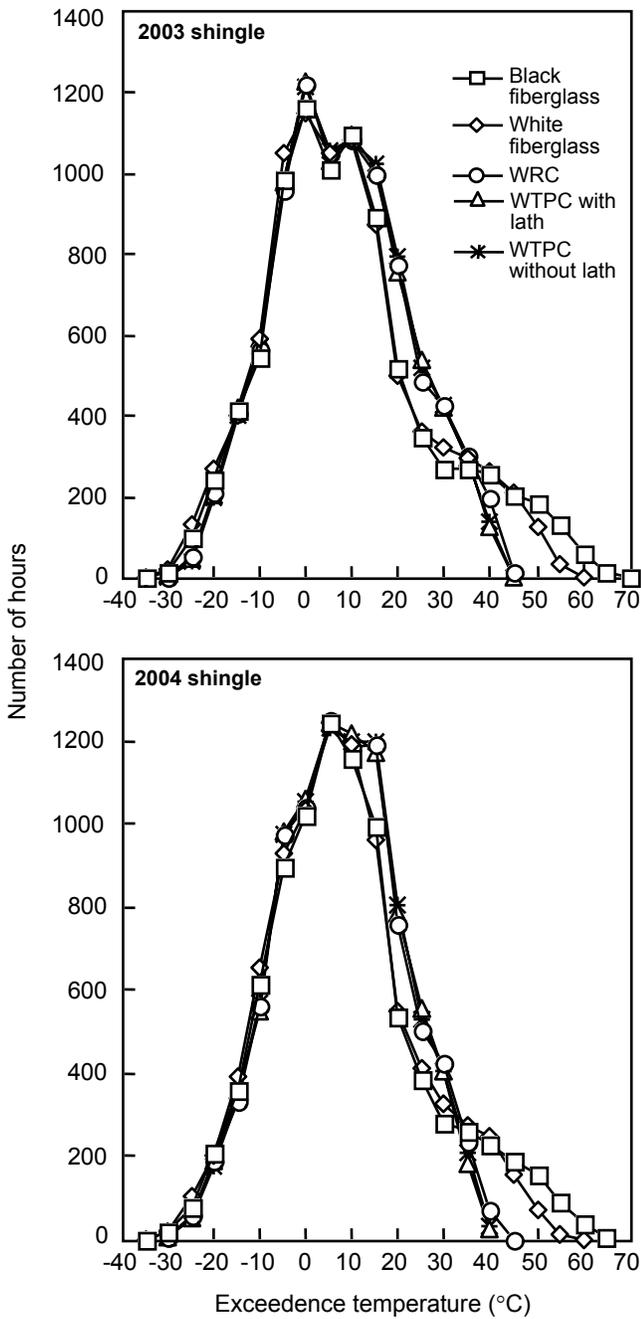
**Figure 4—Cumulative temperature histories of WTPC (with and without lath), WRC, and fiberglass shingles exposed from January to December in 2003 and 2004 near Madison, Wisconsin.**
