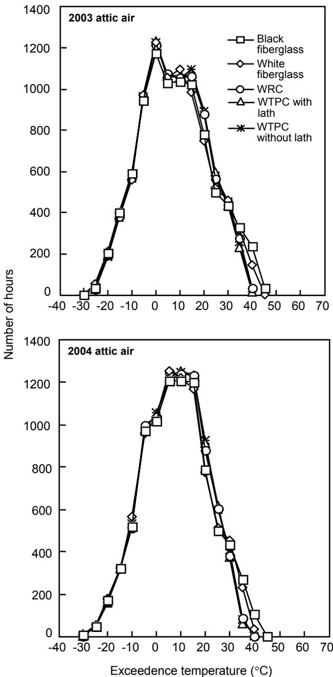
**Figure 8—Cumulative temperature histories of attic air temperature in structures made with various types of shingles.**
