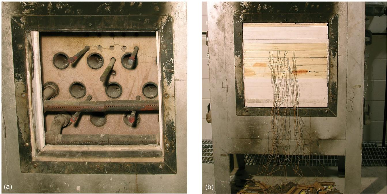
**Figure 2. Opening of small vertical furnace (a) without and (b) with a test specimen in place.**
