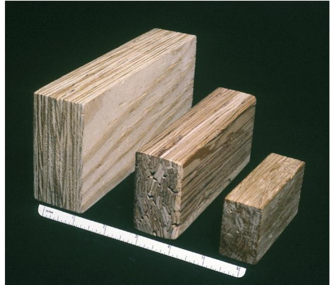
Figure 1. Examples of types of composite lumber products tested in this study: (left to right) laminated veneer lumber, parallel strand lumber, and laminated strand lumber.
