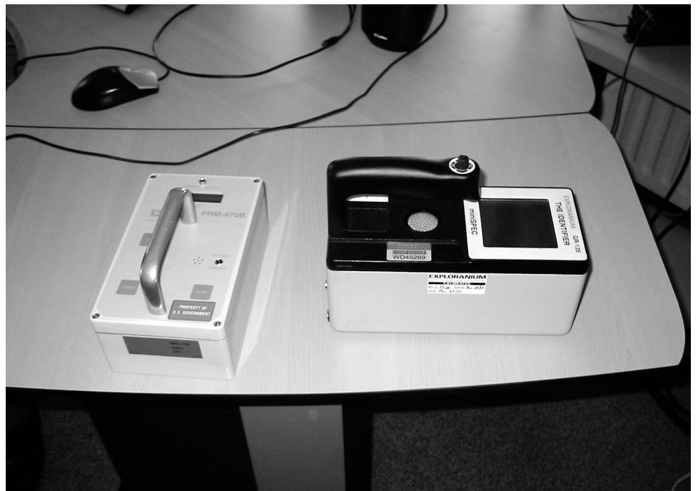
Figure 7: A Handheld Gamma Radiation Detector and a Radioactive Isotope Identification Device
