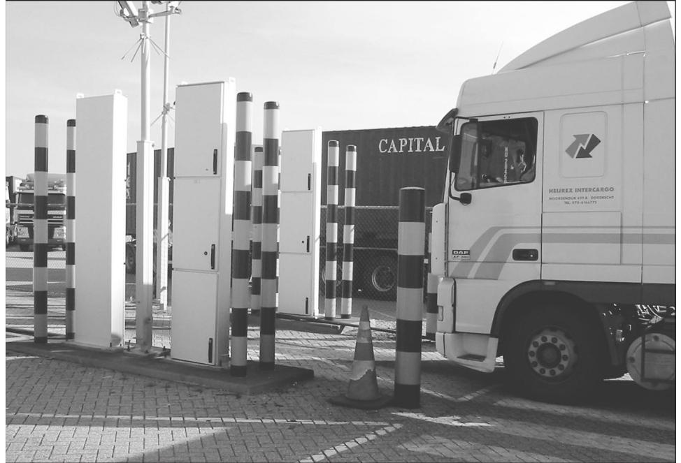
Figure 2: Truck Passing through a Radiation Portal Monitor in Rotterdam, the Netherlands
