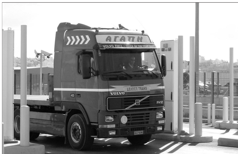
Figure 3: Truck Passing through a Radiation Portal Monitor in Piraeus, Greece
