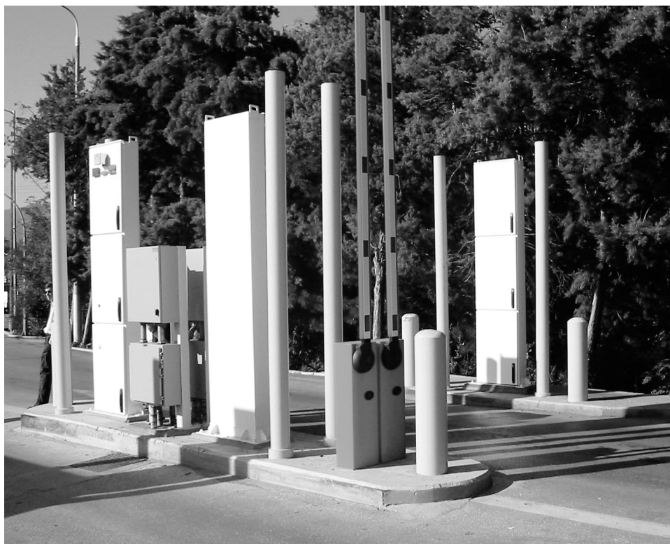
Figure 6: Radiation Portal Monitors at a Northern Greek Border Crossing
