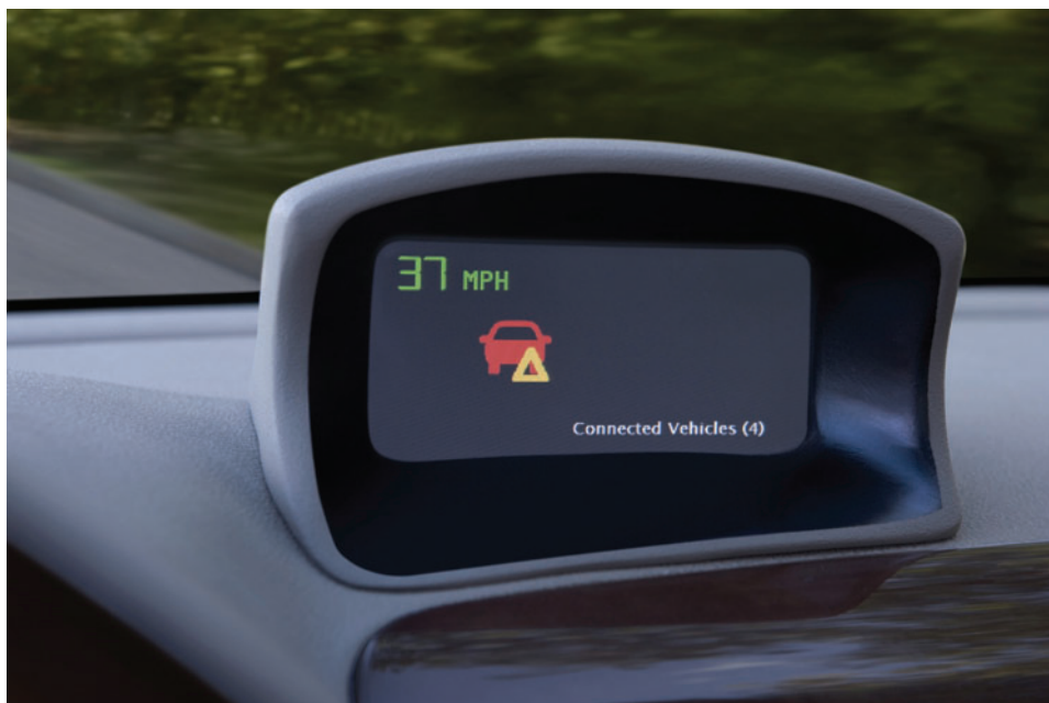
Figure 18: Screen with V2V Icon Warning of a Stopped Vehicle in the Road Ahead
