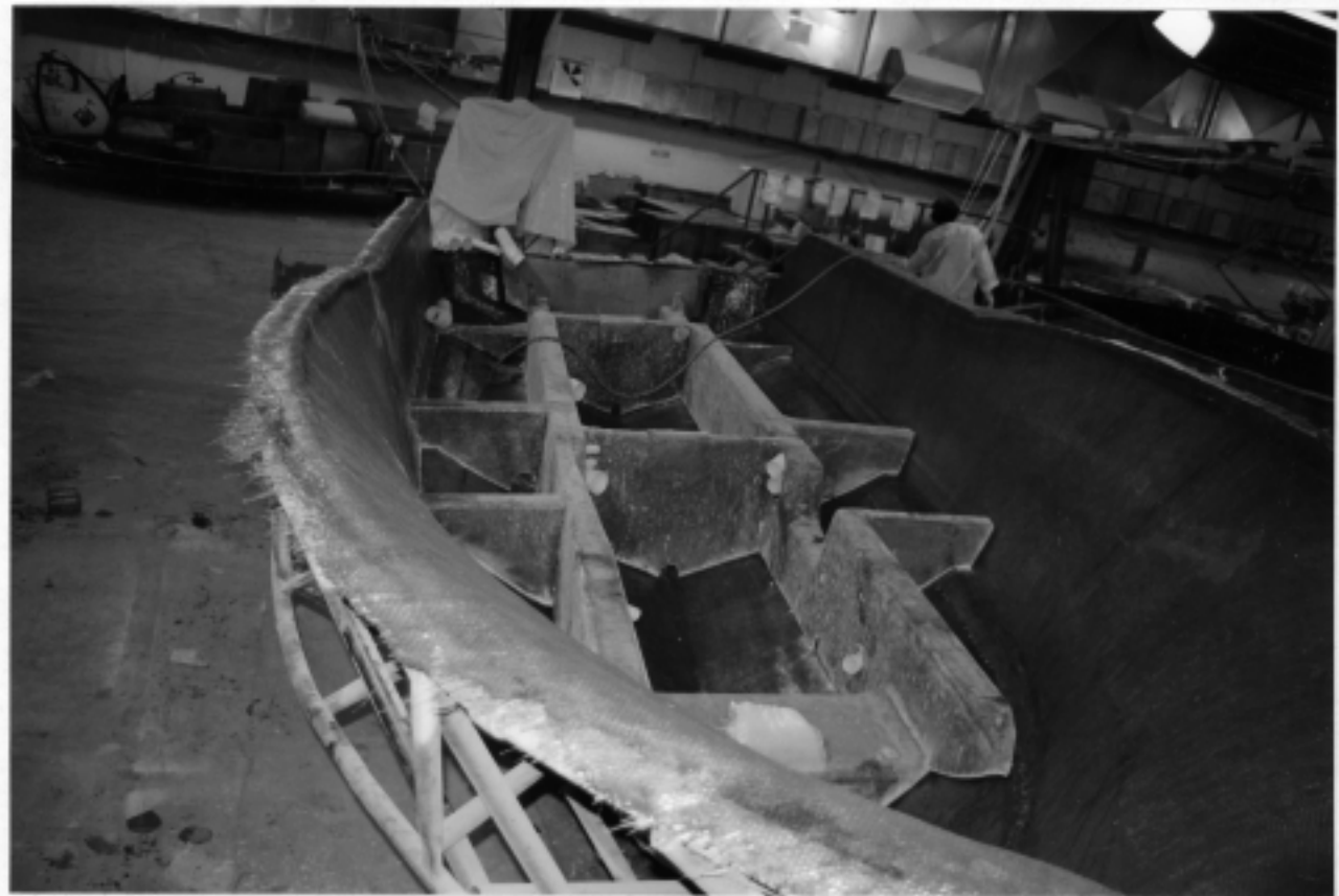
POLAR 27 CENTER CONSOLE STRINGER INSTALLATION
